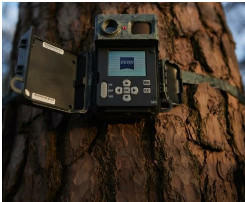
Figure 5: Camera Mounted (Open for Alignment). This image demonstrates the camera mounted on a tree with its front cover open, allowing for precise alignment using the internal display.
