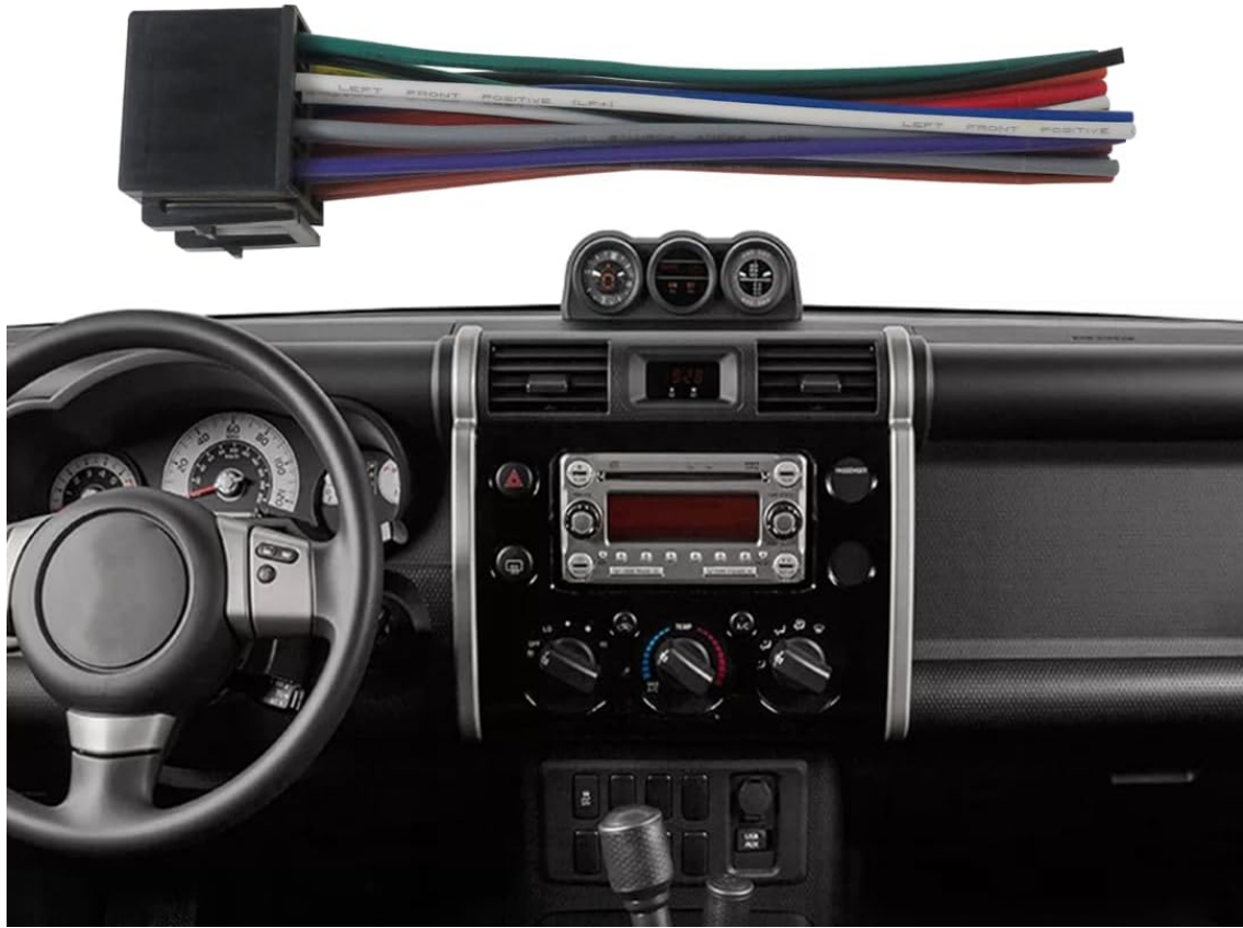
Image 3.1: The car radio stereo harness with its standard color-coded wires, shown above a car's dashboard. This illustrates how the harness plugs into the factory system without cutting wires, simplifying installation.
