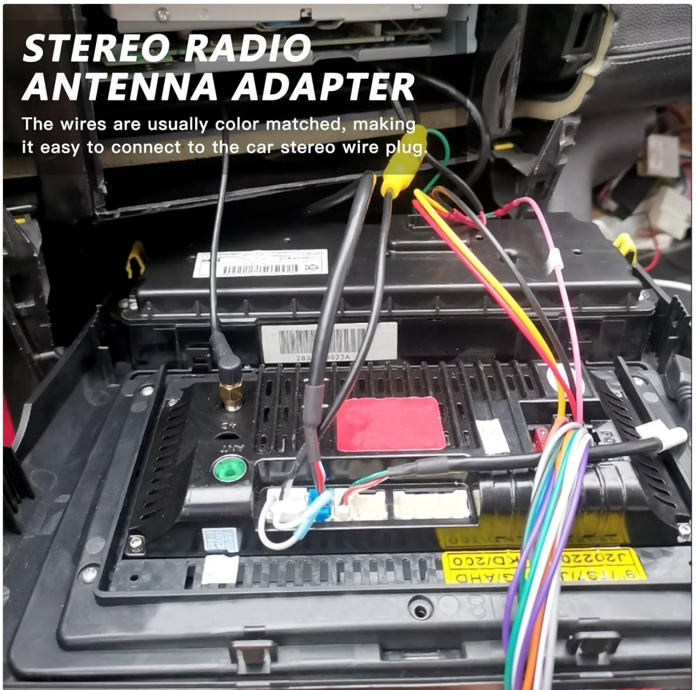
Figure 3: An example of a car stereo installation in progress, demonstrating how the wire harness connects to the vehicle's existing wiring. This visual aids in understanding the physical connection process.
