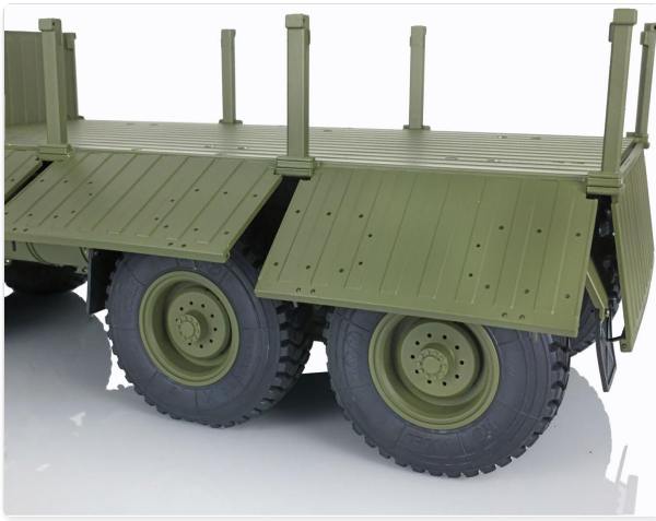
Image 3.3: Rear view demonstrating the adjustable truck bed side panels.
