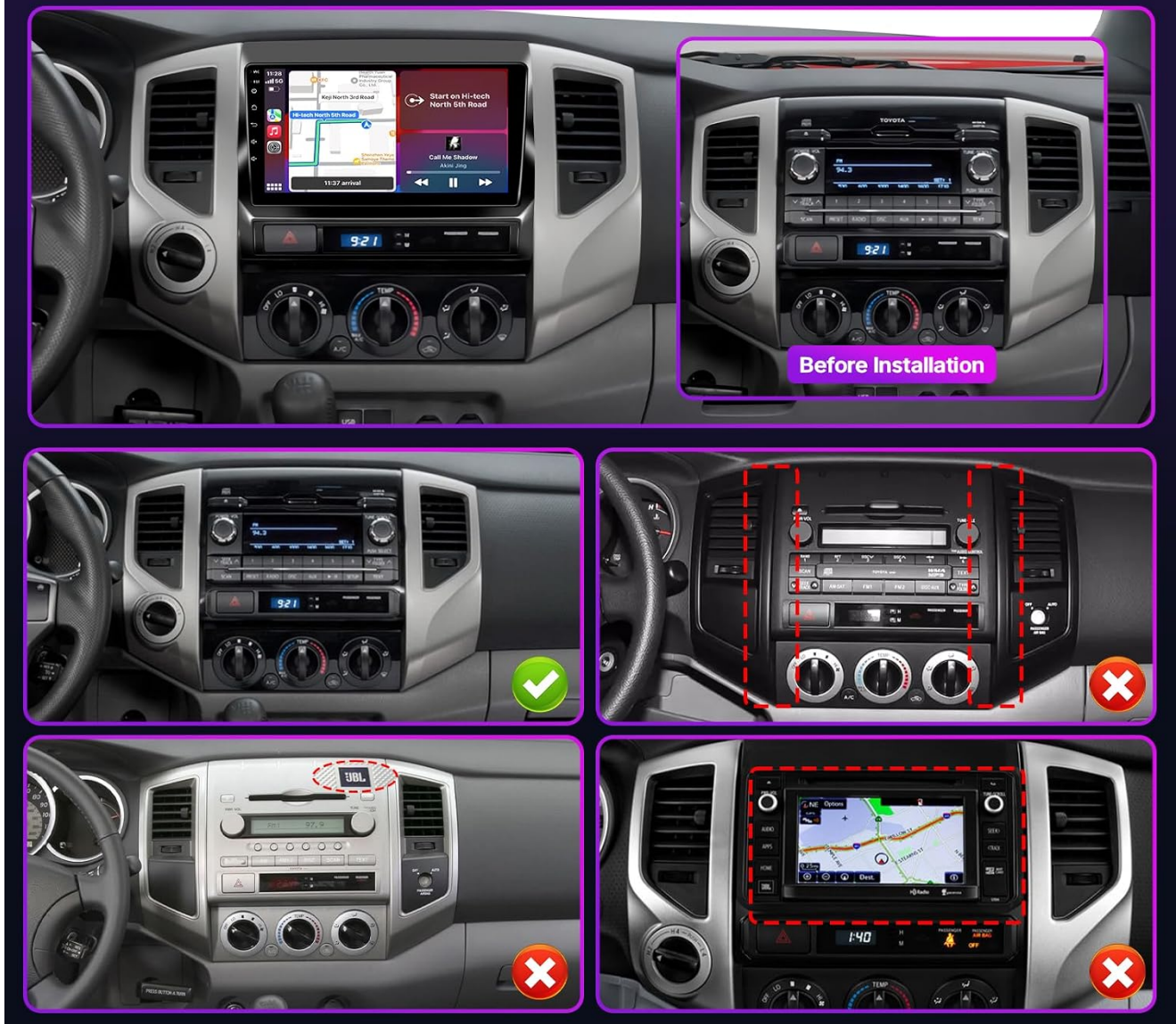
Image 3.1: Visual guide illustrating compatible and incompatible dashboard configurations for installation.
