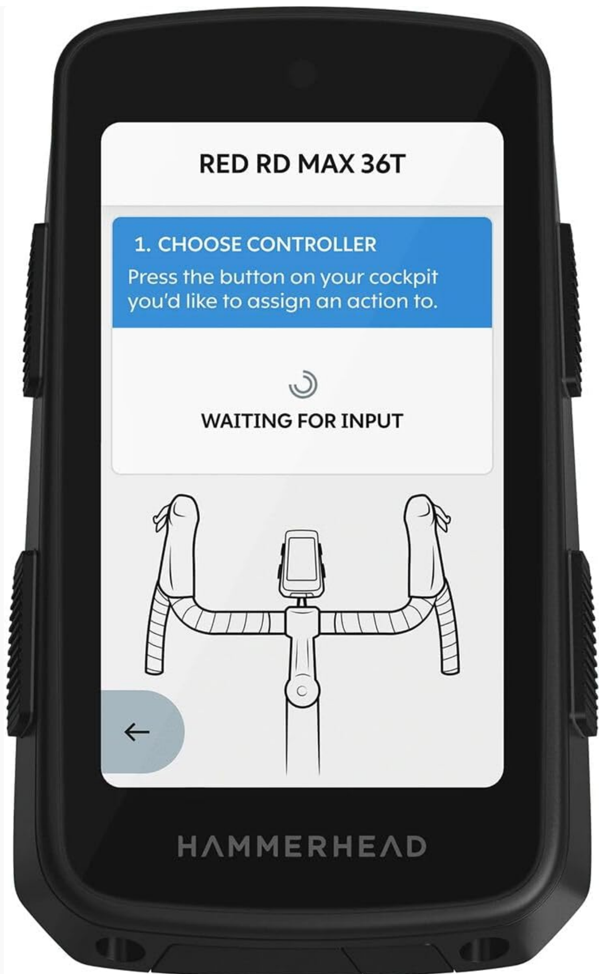
Figure 3.1: The Karoo device displaying the controller setup screen, prompting the user to press a button on their cockpit.
