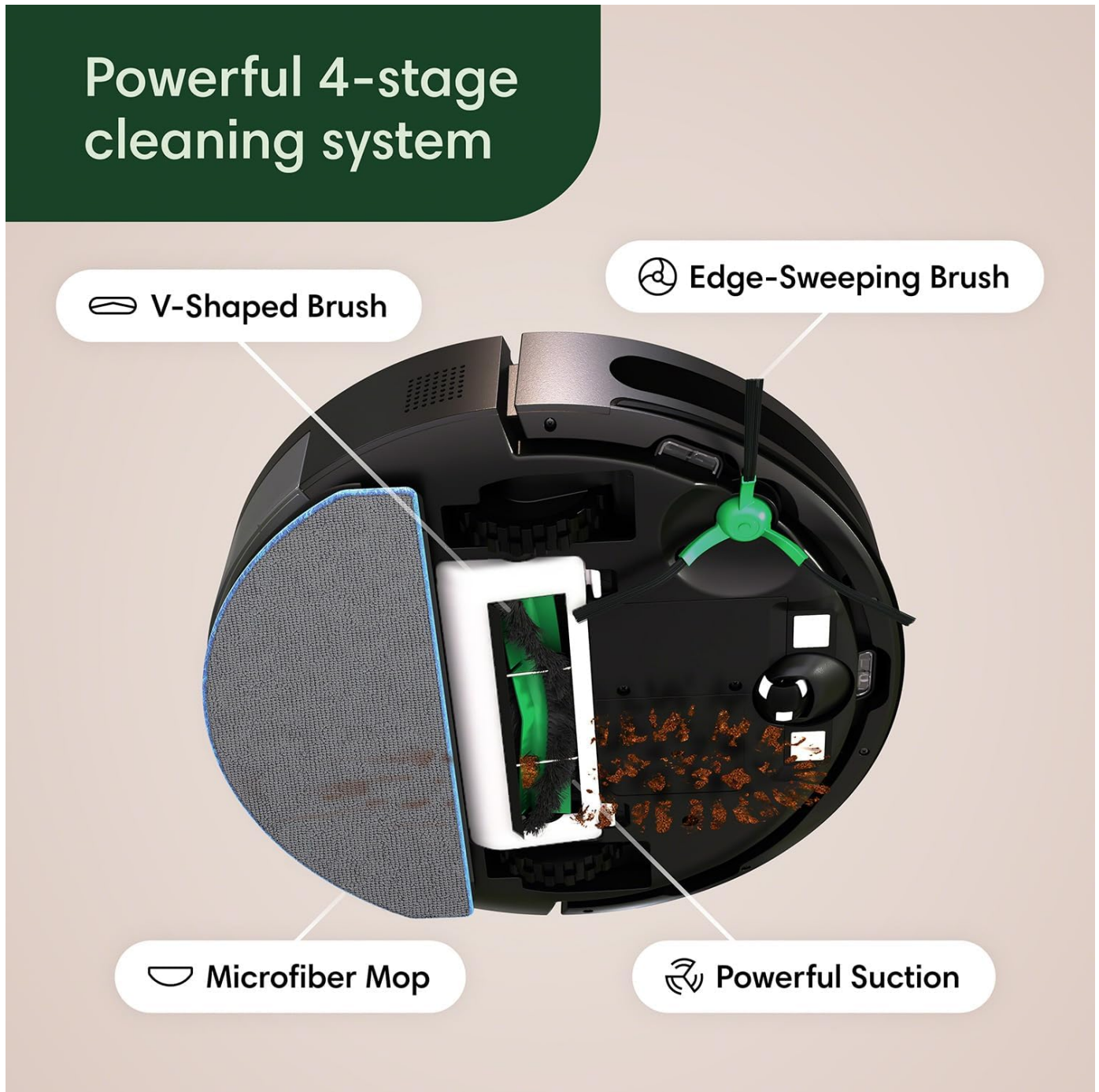
Figure 2: Components of the 4-stage cleaning system, including the V-shaped brush, Edge-Sweeping Brush, powerful suction, and microfiber mop.
