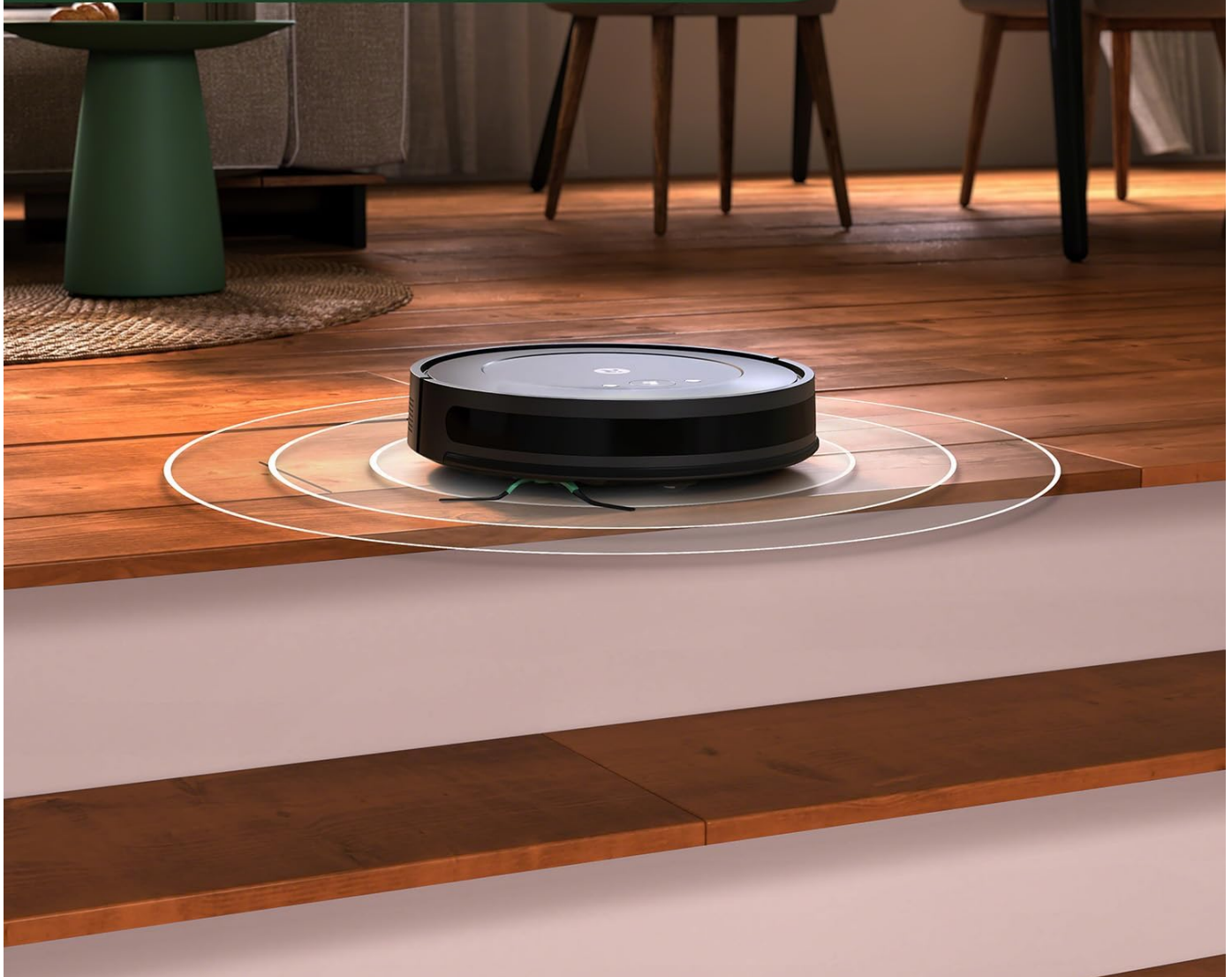
Figure 4: The robot's sensors detect the edge of stairs, preventing it from falling.
