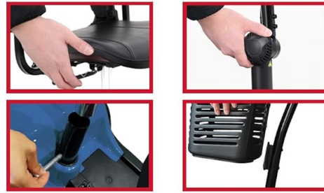
Figure 1: Quick and efficient assembly of the M1 Lite scooter. Components include the basket, battery box, and seat with armrests.
