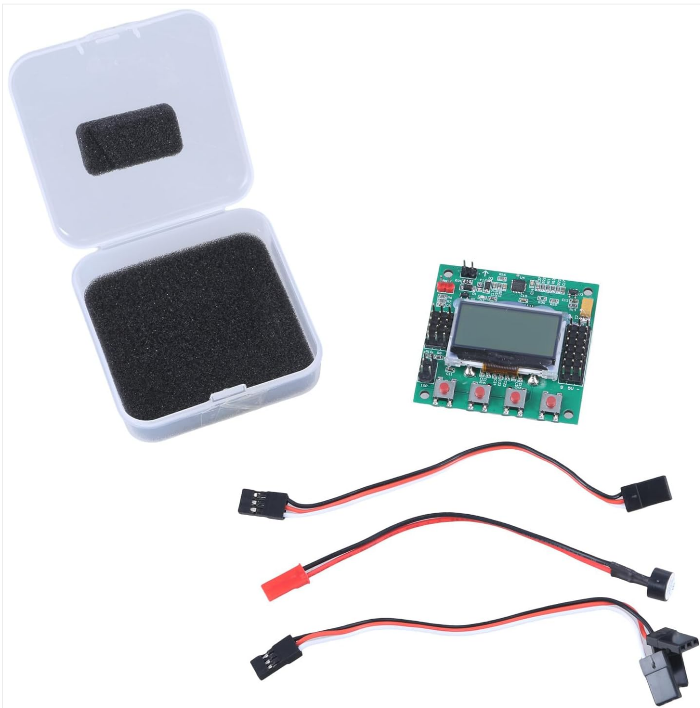
Image: The KK 2.1.5 Flight Control Board shown with its included accessories, including connection cables and a protective case.
