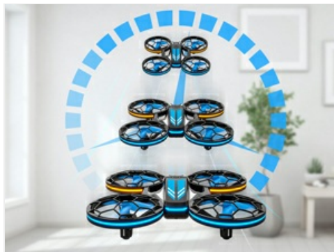
Image: Diagram showing the drone's movement in Headless Mode, where direction is relative to the remote control.
