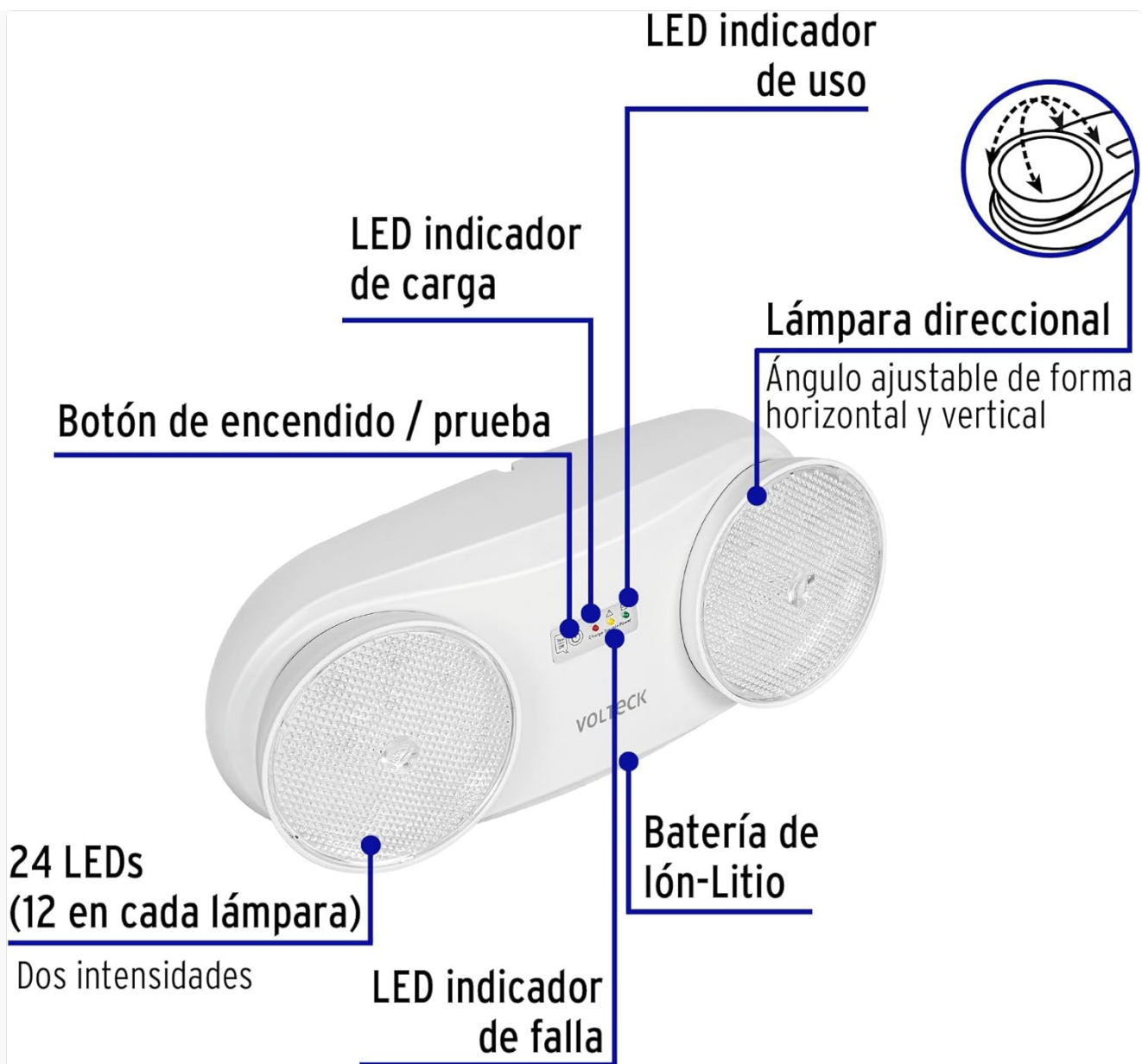
Figure 3.1: Lamp Components. This image shows the Volteck LAE-24D emergency lamp with various parts labeled. Key components include the On/Test Button, Charge Indicator LED, In-Use Indicator LED, Fault Indicator LED, Directional Lamps (24 LEDs total, 12 per lamp), and the Lithium-Ion Battery. The directional lamps can be adjusted horizontally and vertically.
