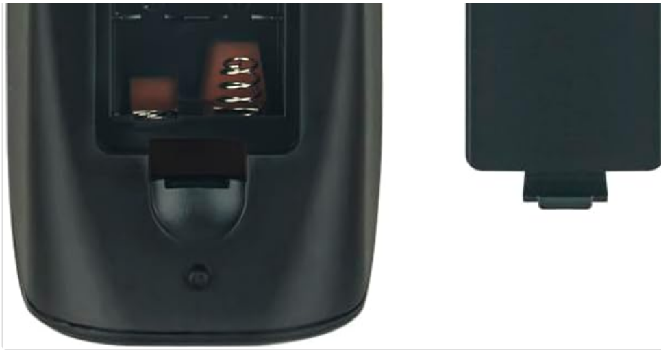
Image 5: Rear view of the remote control with the battery compartment open, revealing the battery slots.
