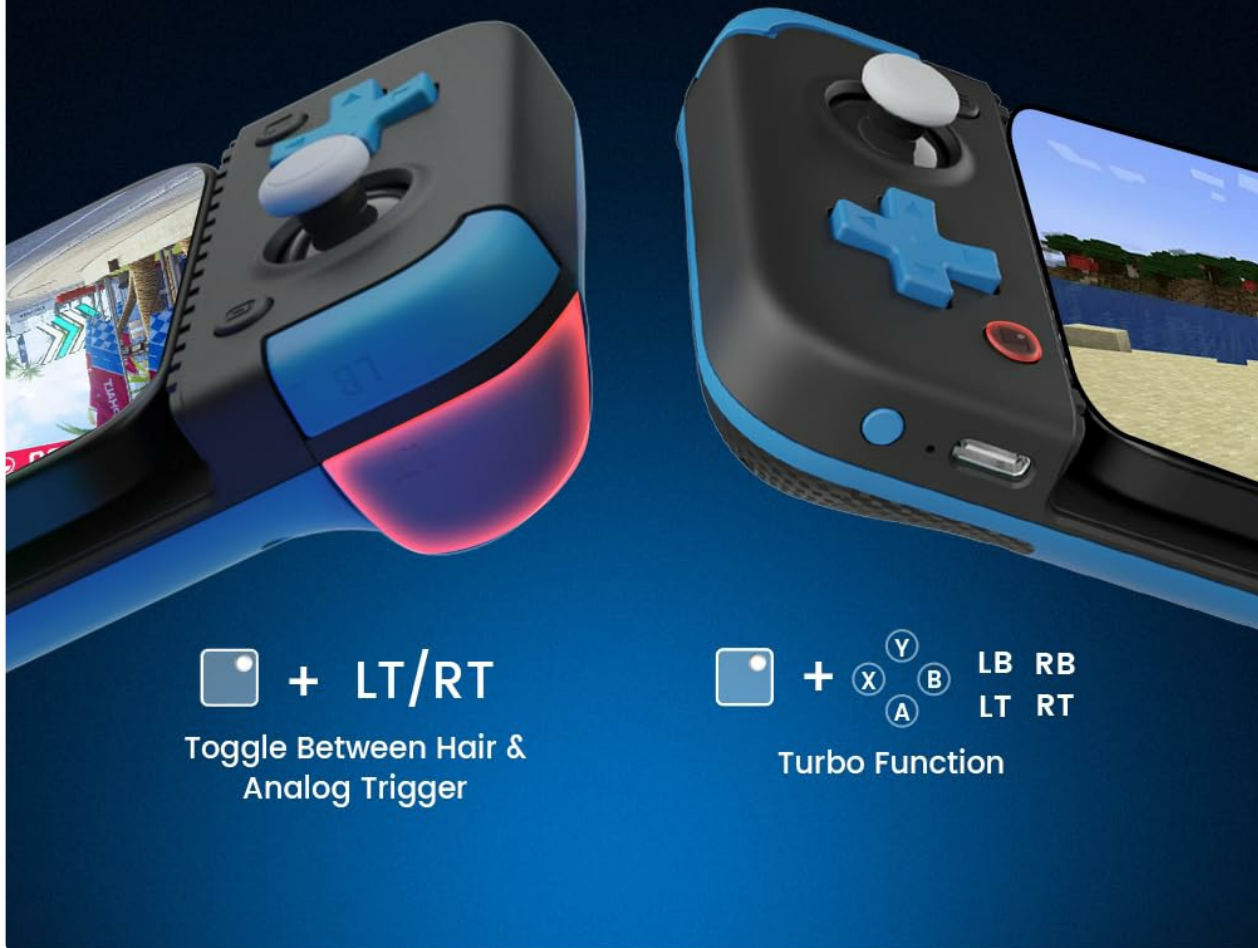
Image 7: Trigger mode toggle and Turbo function activation.
