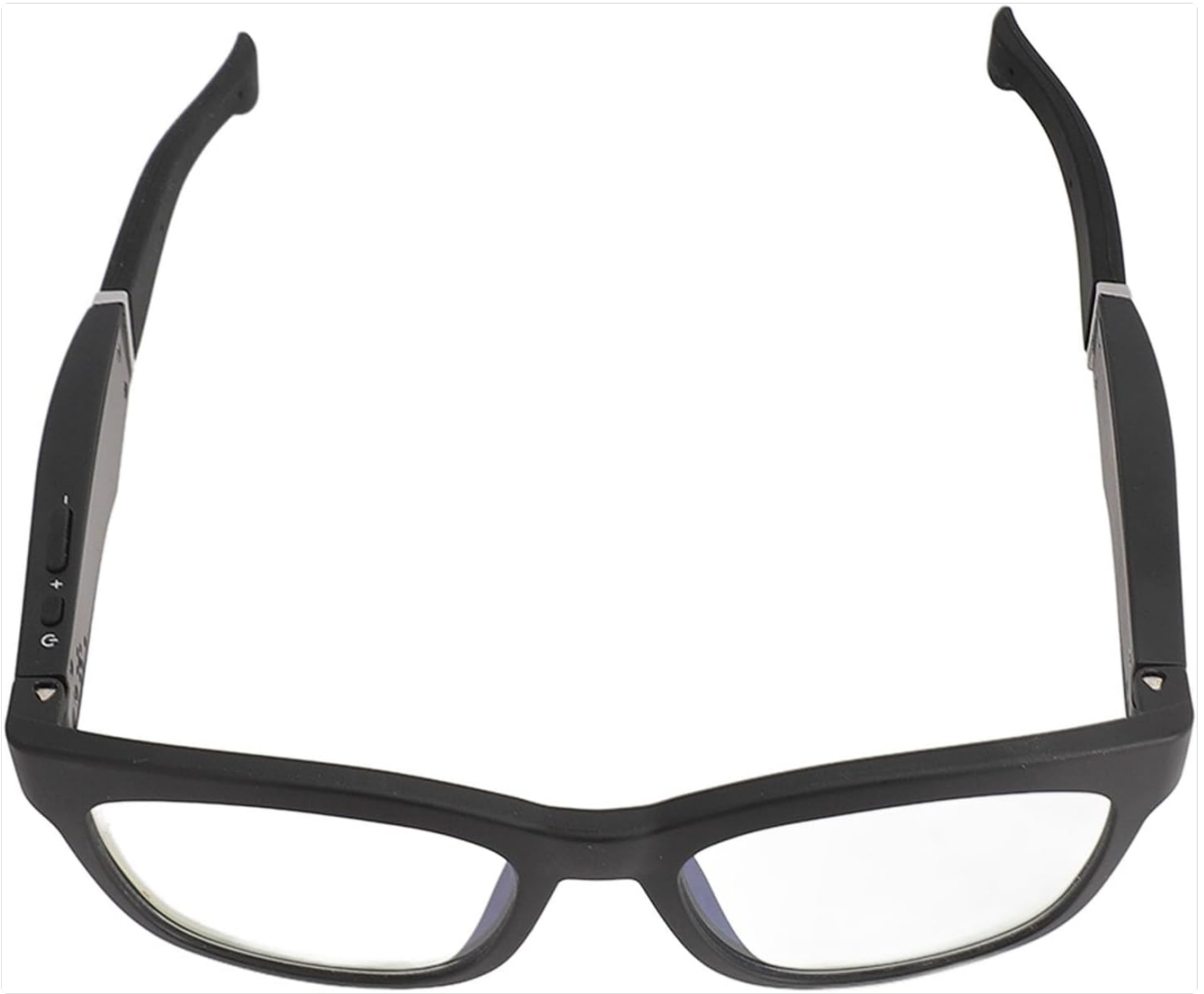
Top view of the right temple, highlighting the control buttons.
