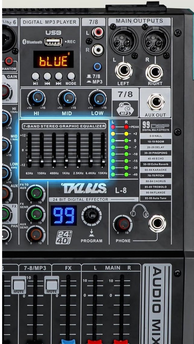
Image: Close-up of the mixer's DSP effects section, showing the program knob, digital display, and a list of 99 available effects.
