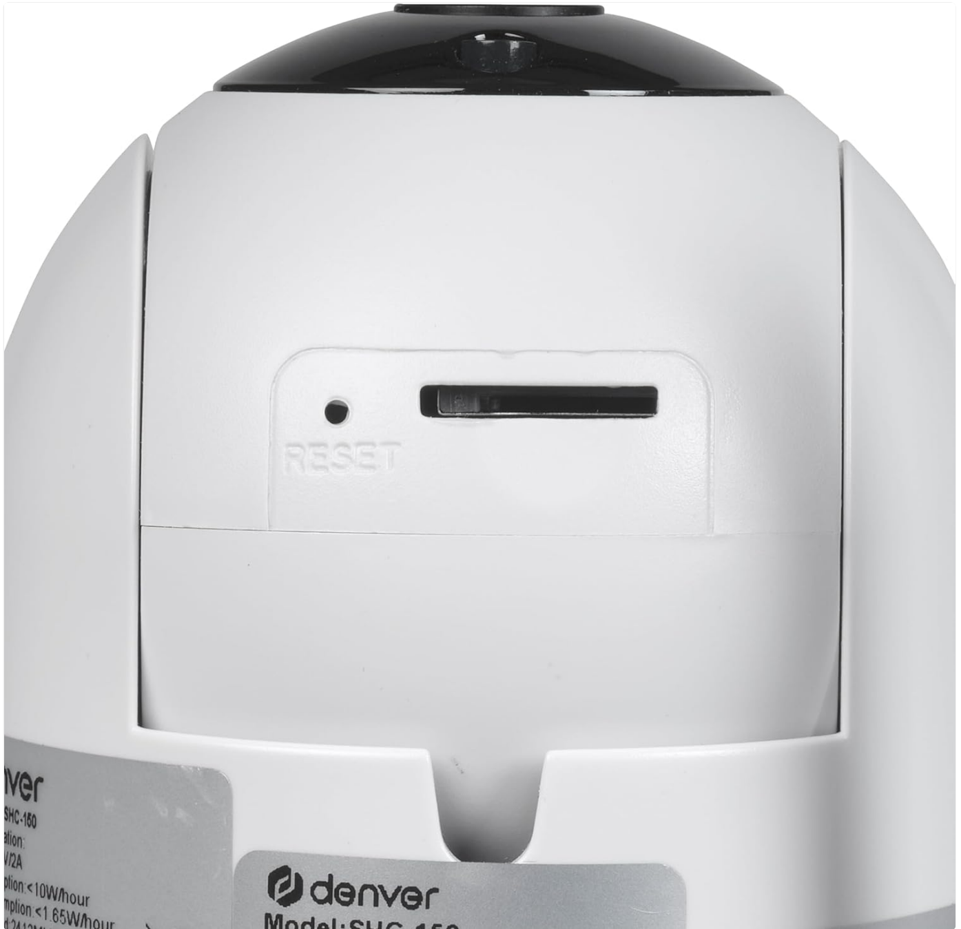
Figure 4.3: Rear view of the Denver IIC-172 camera, highlighting the recessed reset button and the MicroSD card slot.
