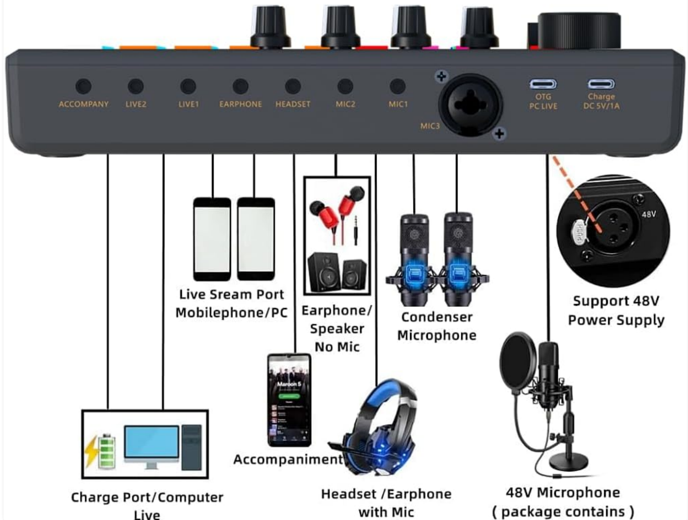
Figure 4: K800 Device Connection Diagram
