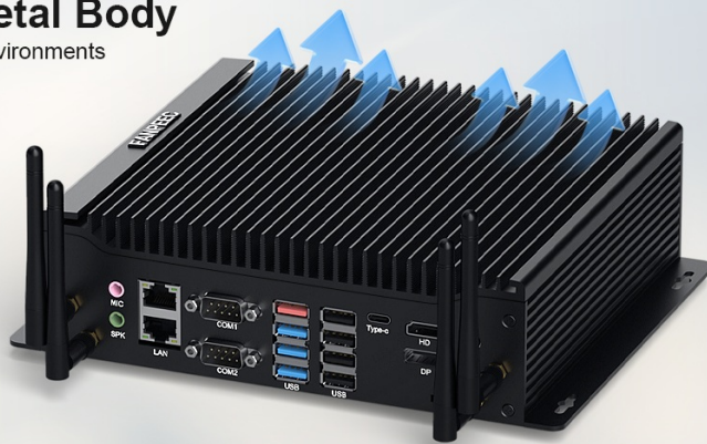
Figure 4.2: This image illustrates the fanless design and metal body of the FANPEEC Mini PC, emphasizing its dust-proof, moisture-proof, shockproof, and wide operating temperature range (-10~55°C) capabilities for stable operation in harsh environments.
