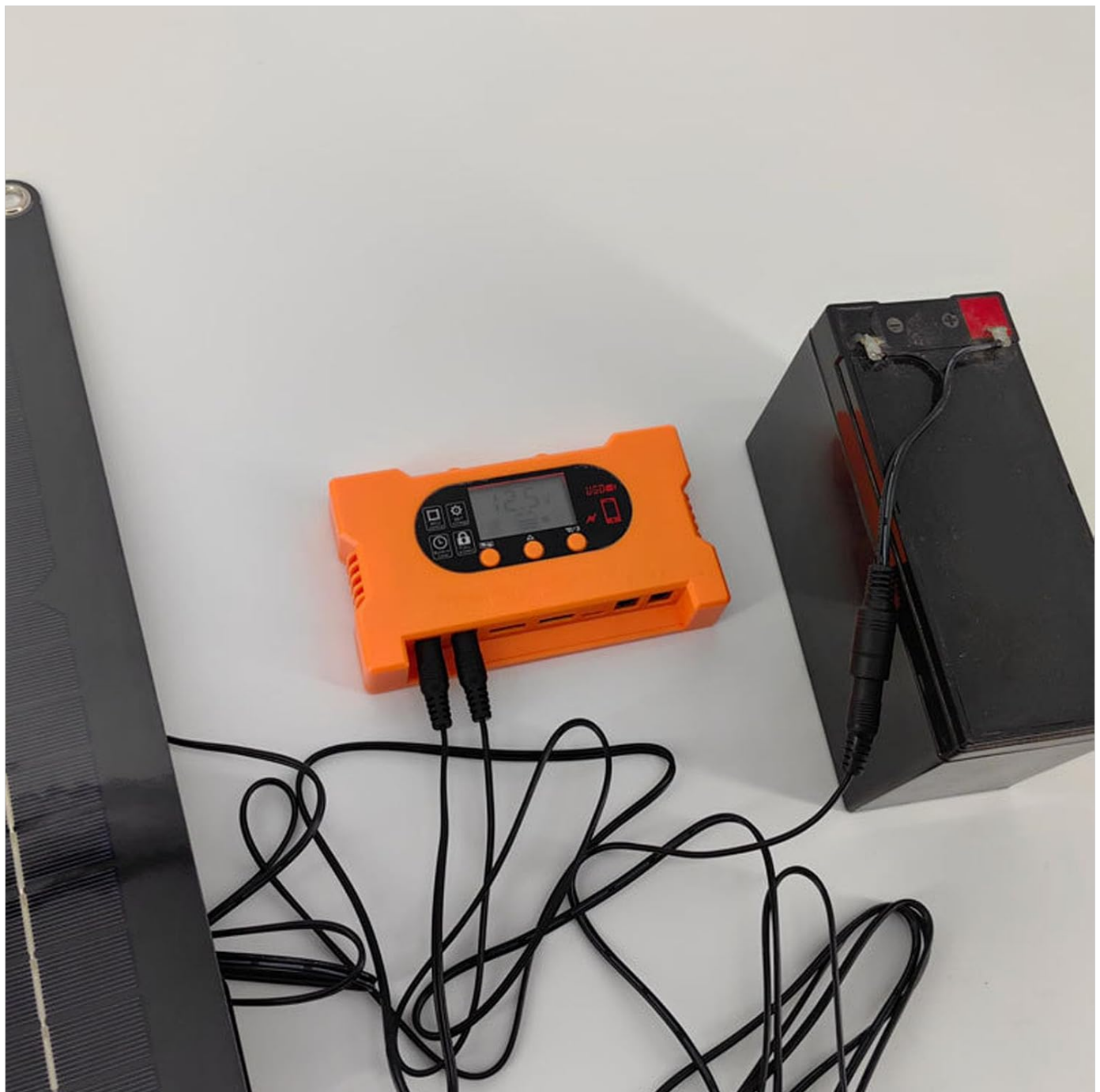
Image: A Topyond solar charge controller is shown connected to a solar panel on the left and a battery on the right, illustrating the correct wiring setup.
