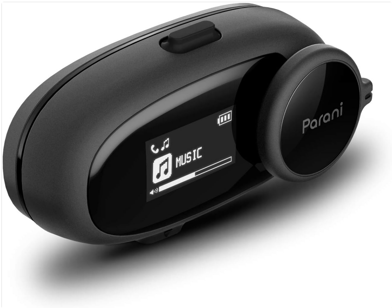
Figure 5: The Parani M10 headset, featuring the Multi-function Button (top) and Jog Dial (right).
