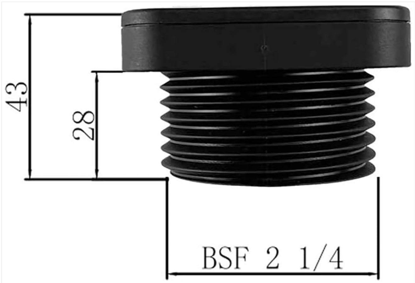
Figure 4.1: Sensor Dimensions (BSF 2 1/4 thread)
