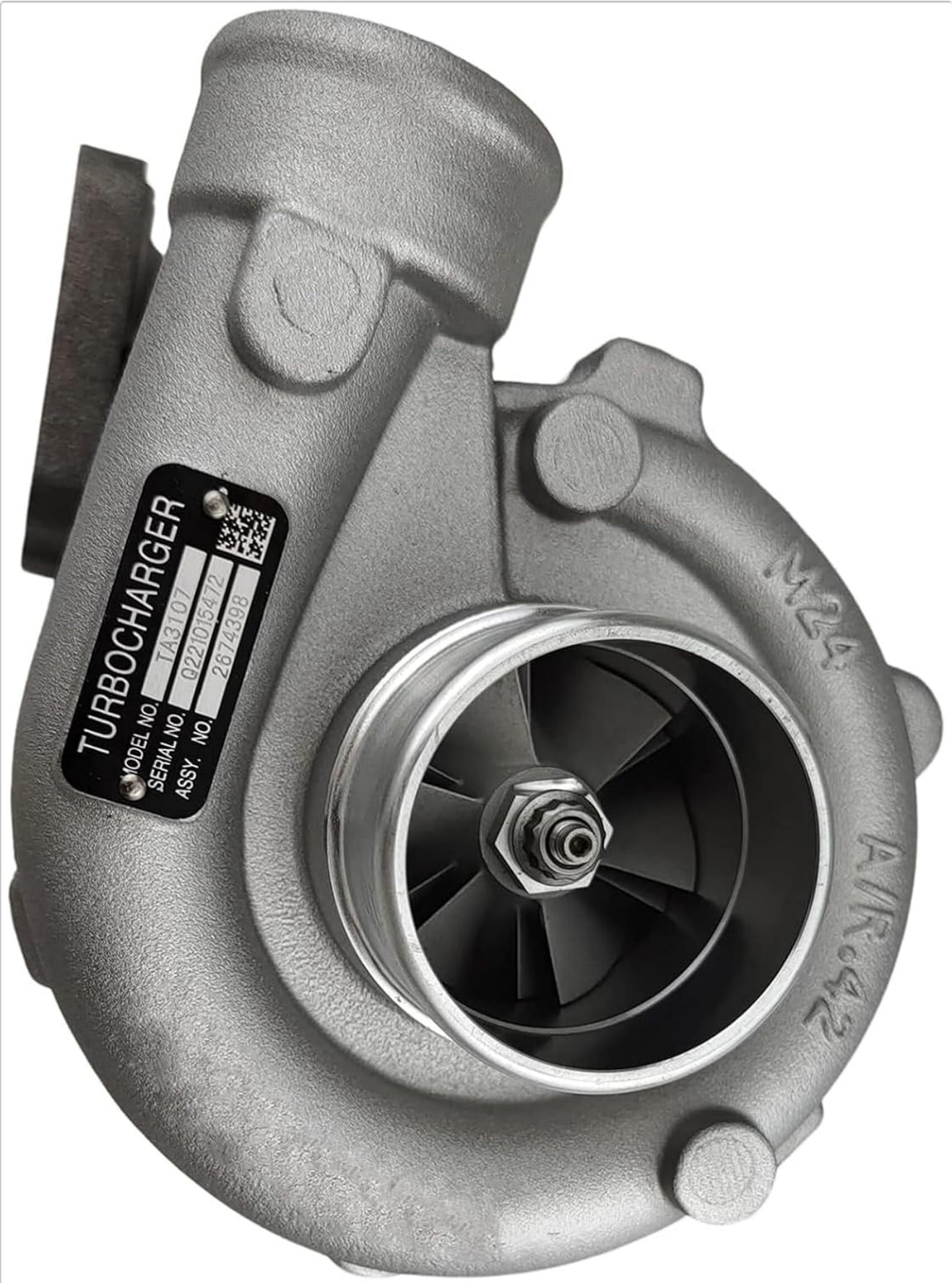
Figure 5.1: View of the compressor wheel, which draws in air and compresses it. Keep the air intake system clean to protect this component.
