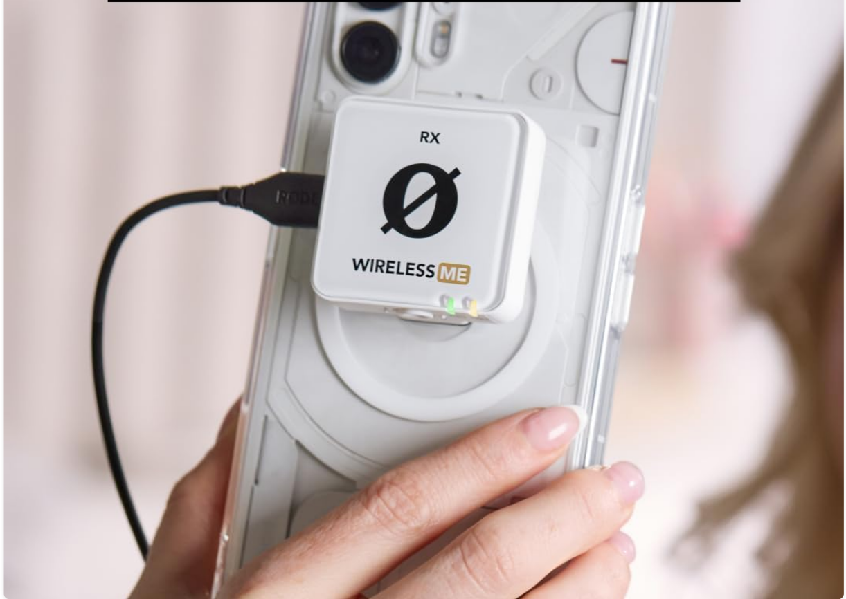
Figure 5: Wireless audio transmission directly to a smartphone using the RØDE Wireless ME receiver.
