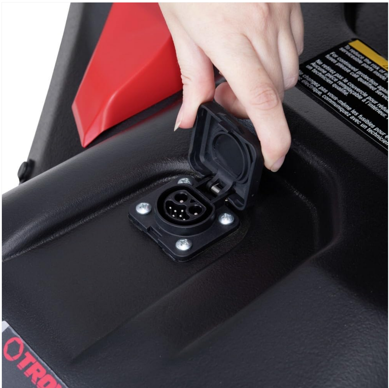
Figure 4: The charging port of the Troy-Bilt TB30E XP with the cover open, showing the multi-pin connector.
