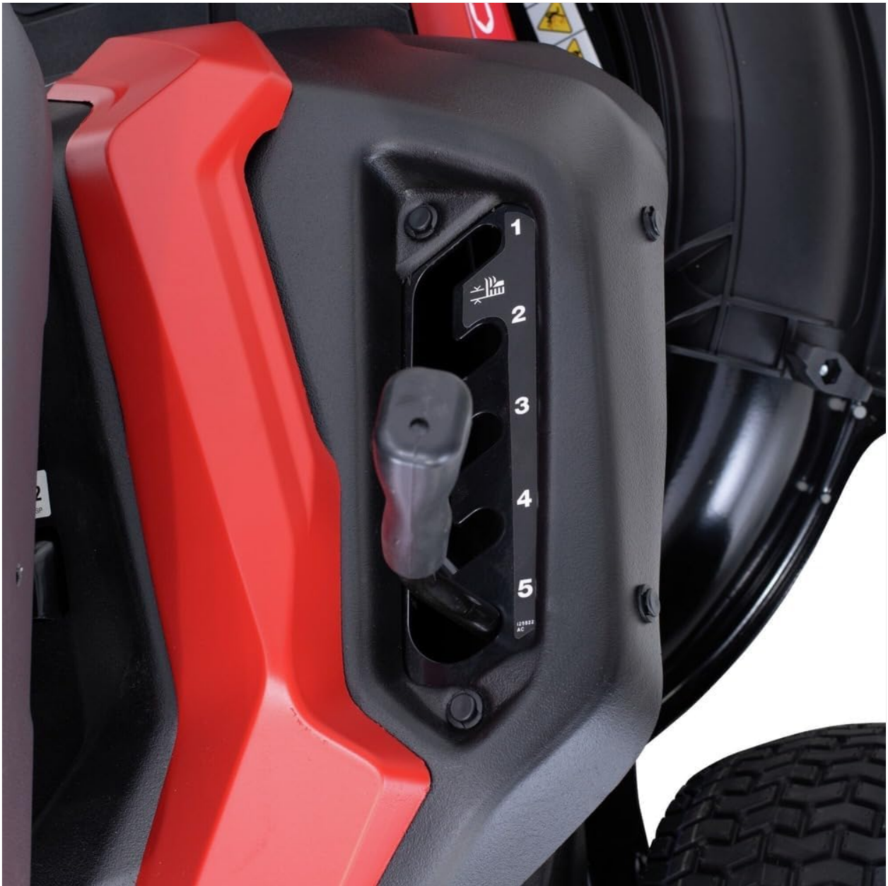
Figure 5: Close-up of the cutting height adjustment lever on the Troy-Bilt TB30E XP, showing numbered settings from 1 to 5.
