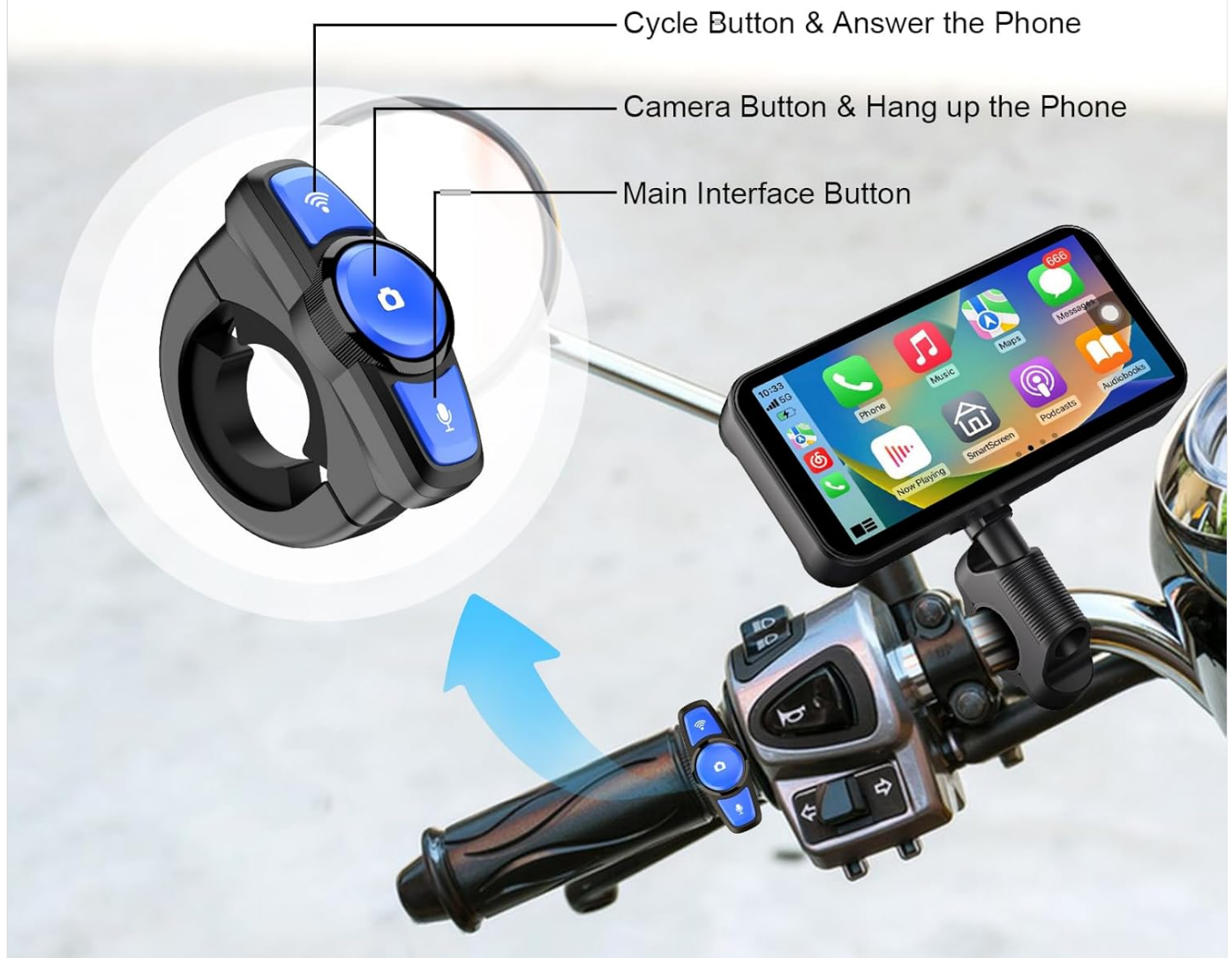
Figure 6: The remote control, illustrating the cycle, camera, and main interface buttons for easy operation.
