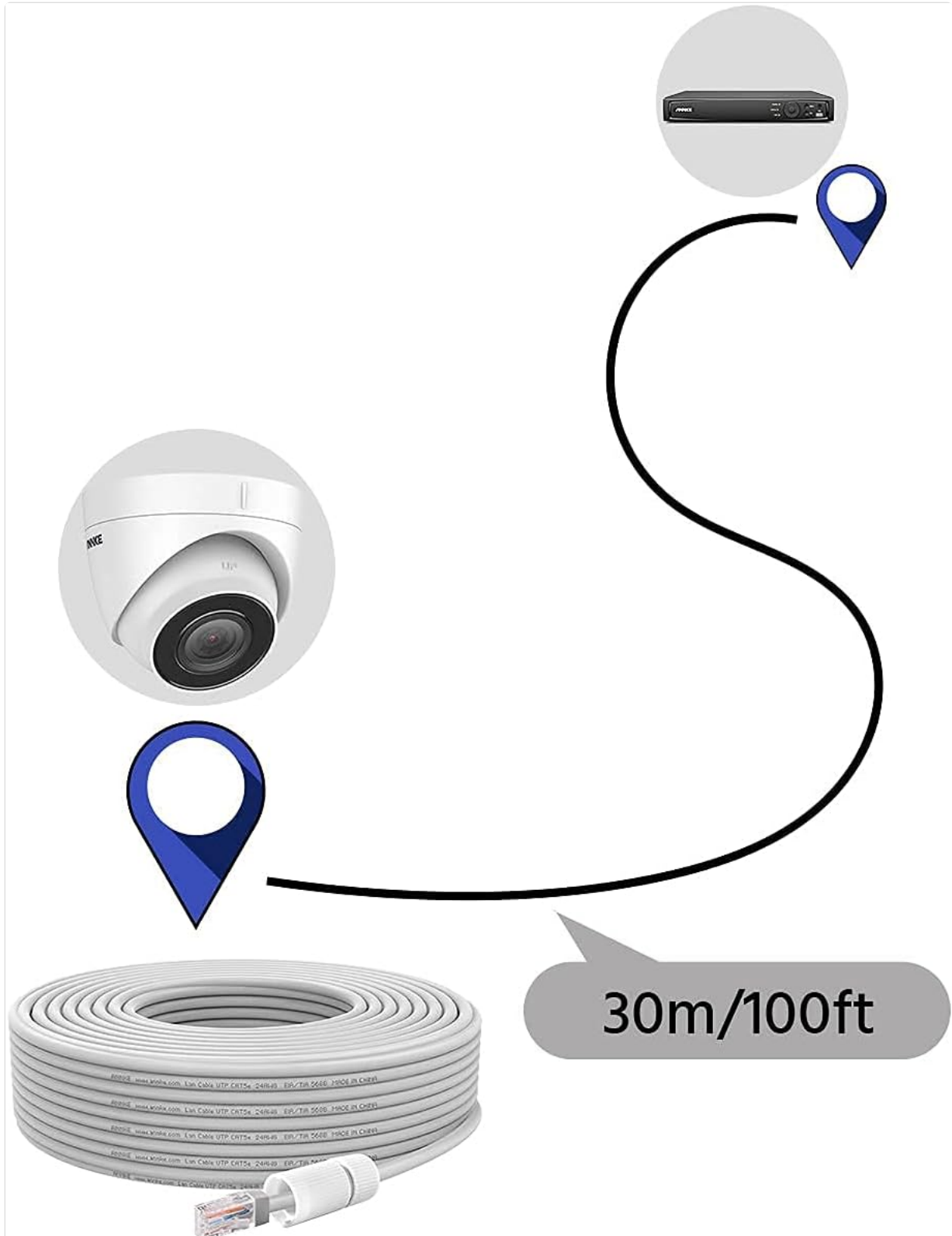
Figure 2: Connection diagram illustrating the PoE camera connected to an NVR using a 30m/100ft Ethernet cable.
