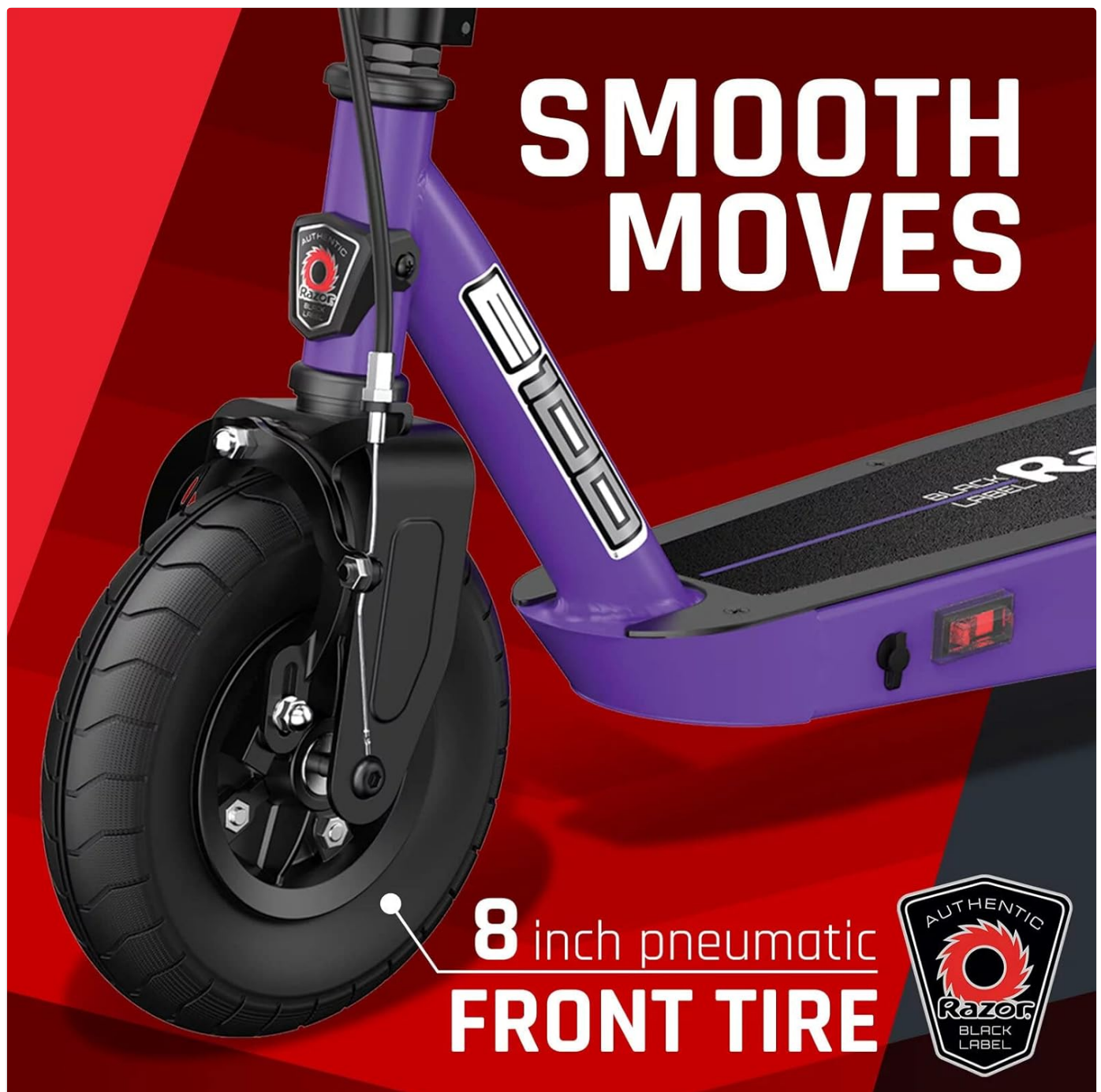
Figure 5: The 8-inch pneumatic front tire, contributing to a smooth and comfortable ride.
