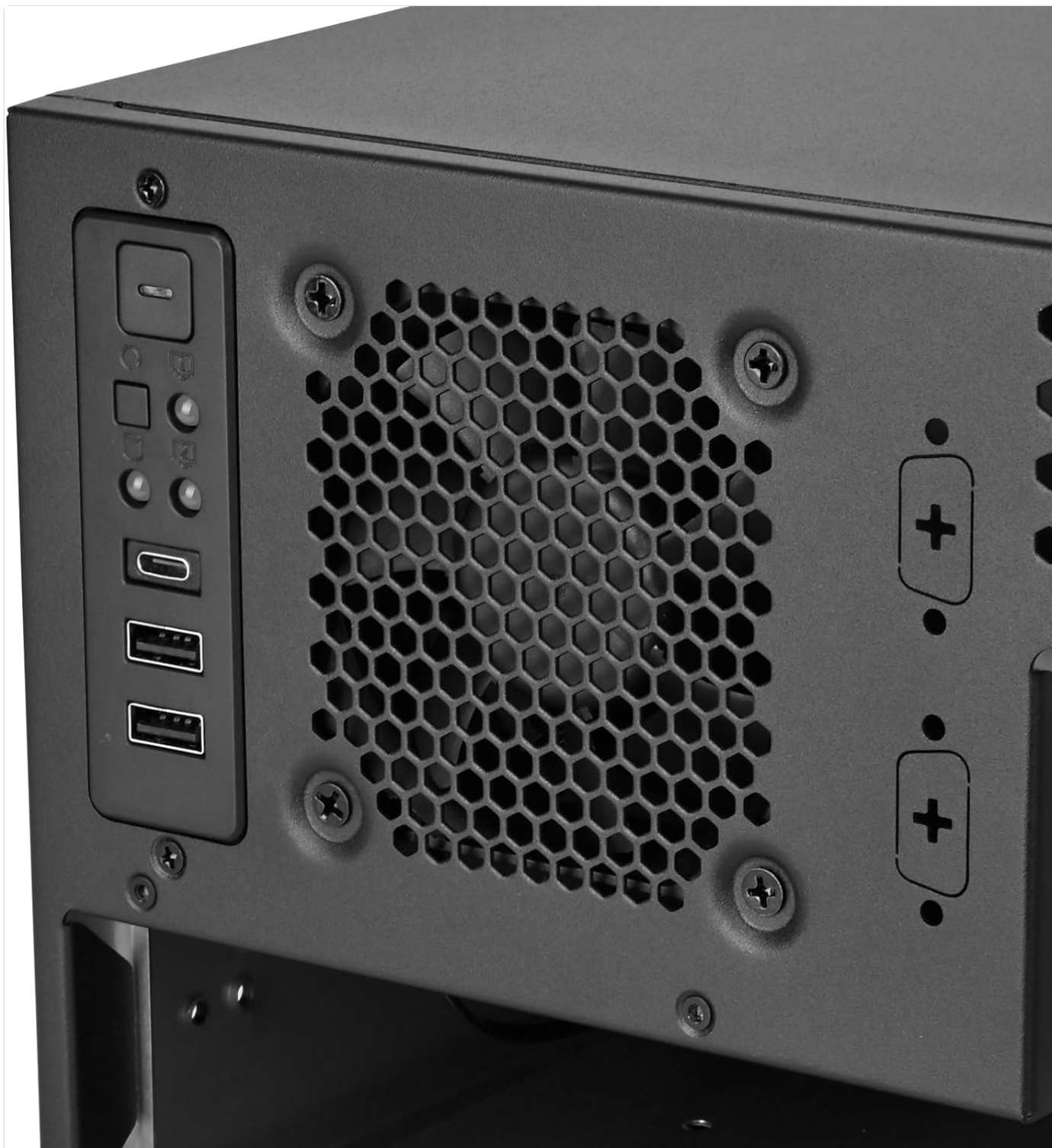
Figure 4.1: Front I/O panel with power button and USB ports.
