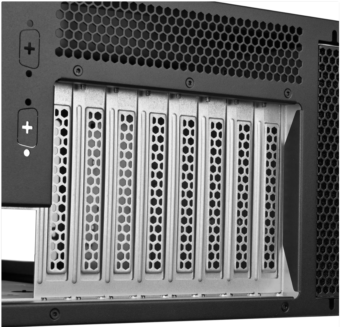
Figure 3.2: Detailed view of the front-facing expansion slots.
