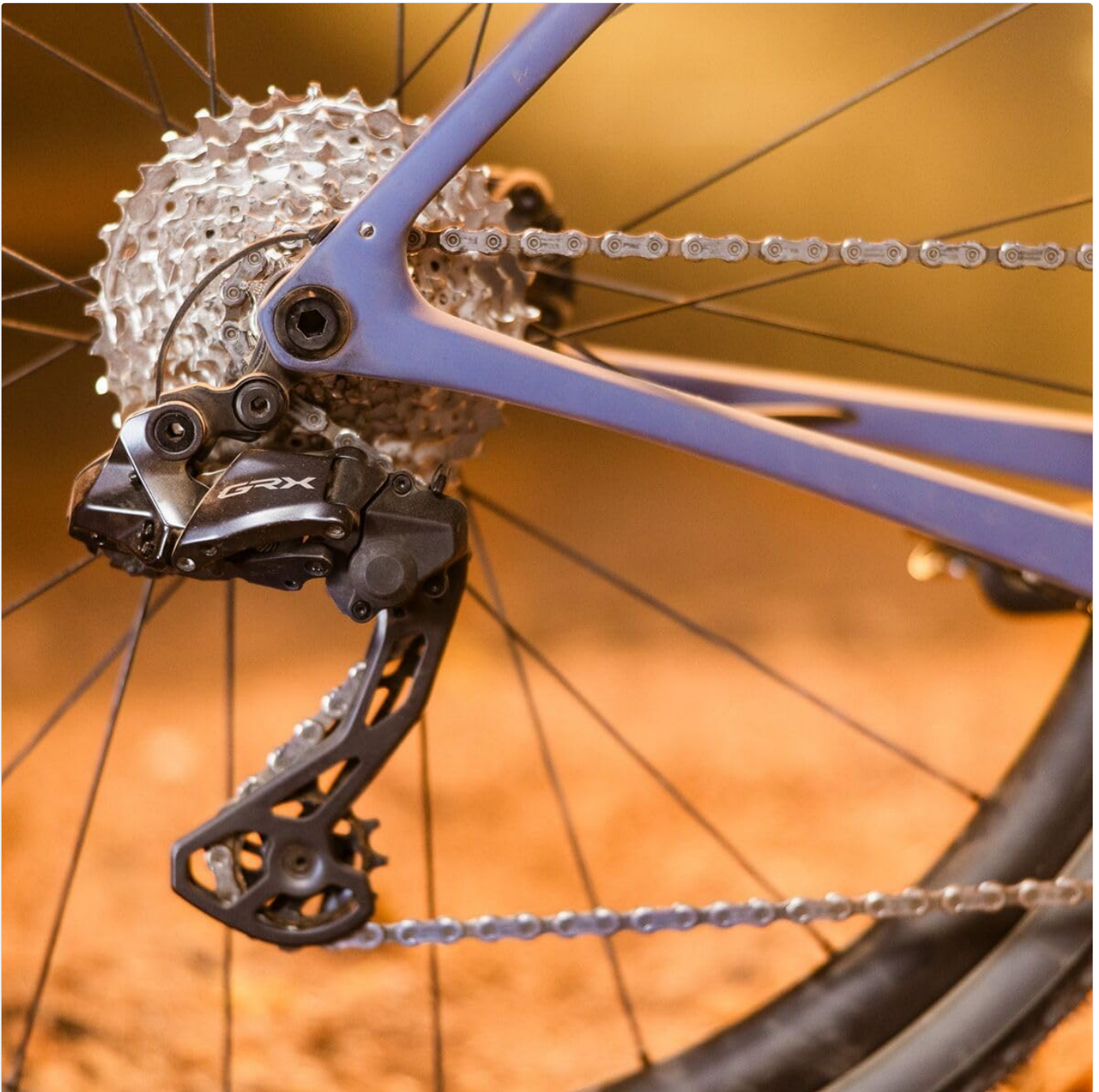
Figure 3: The SHIMANO GRX RD-RX825 Rear Derailleur installed on a bicycle, showing its integration with the cassette and chain. This image demonstrates the derailleur's position relative to the rear wheel and drivetrain components.
