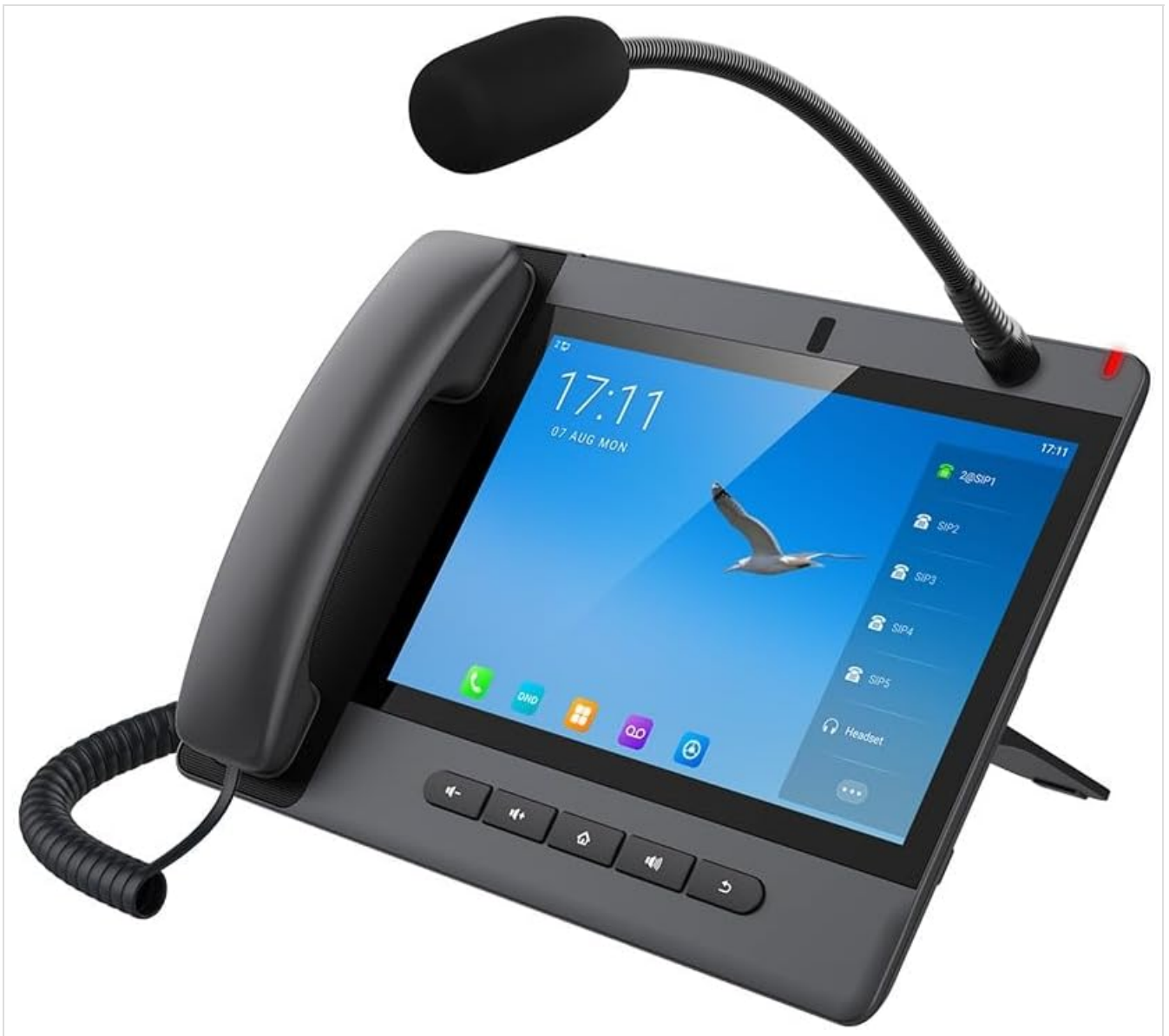
Figure 1: Front view of the Fanvil A320i IP Phone, showing the 10.1-inch touch screen, handset, and gooseneck microphone. The screen displays the time, date, and various application icons.
