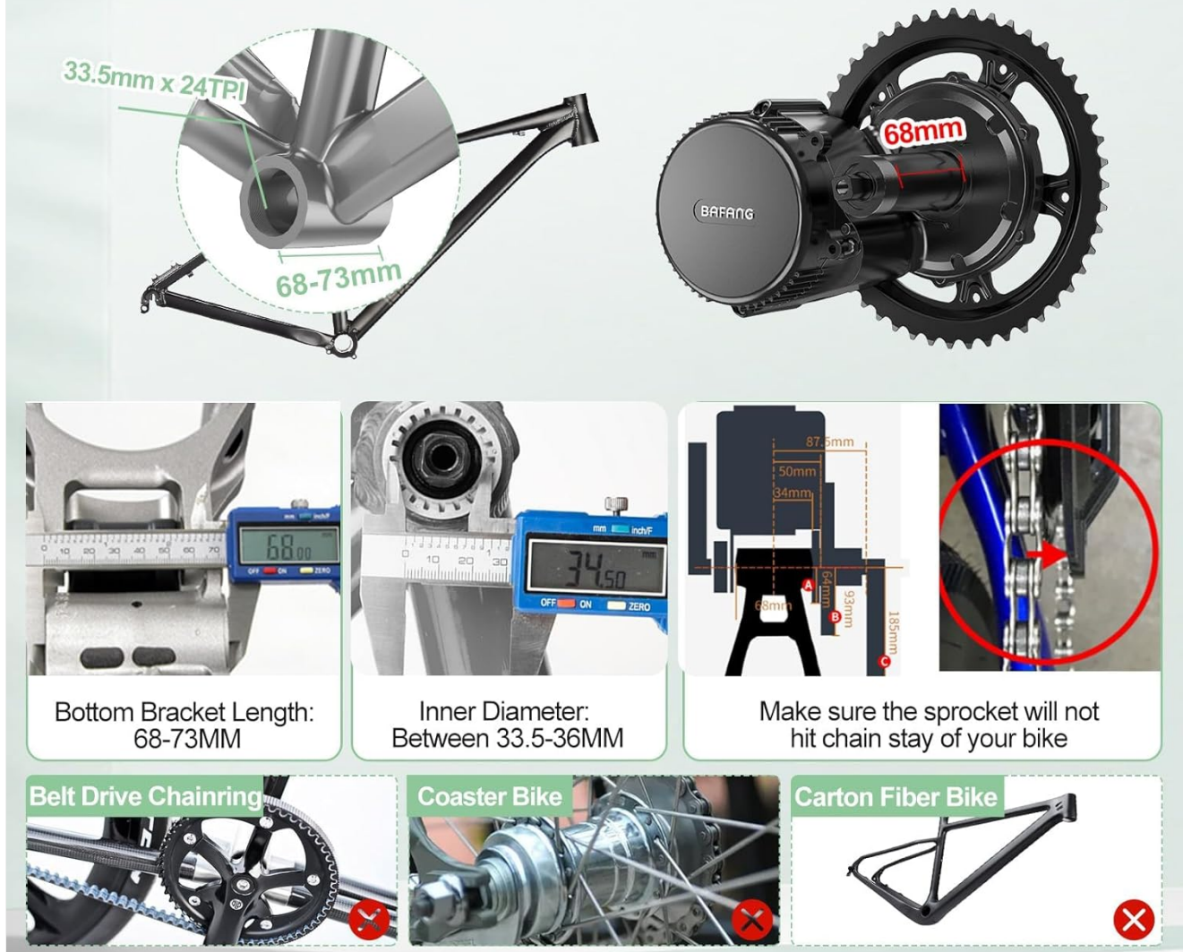
Image 3.1: Guide for checking bike compatibility with the mid-drive motor kit.
