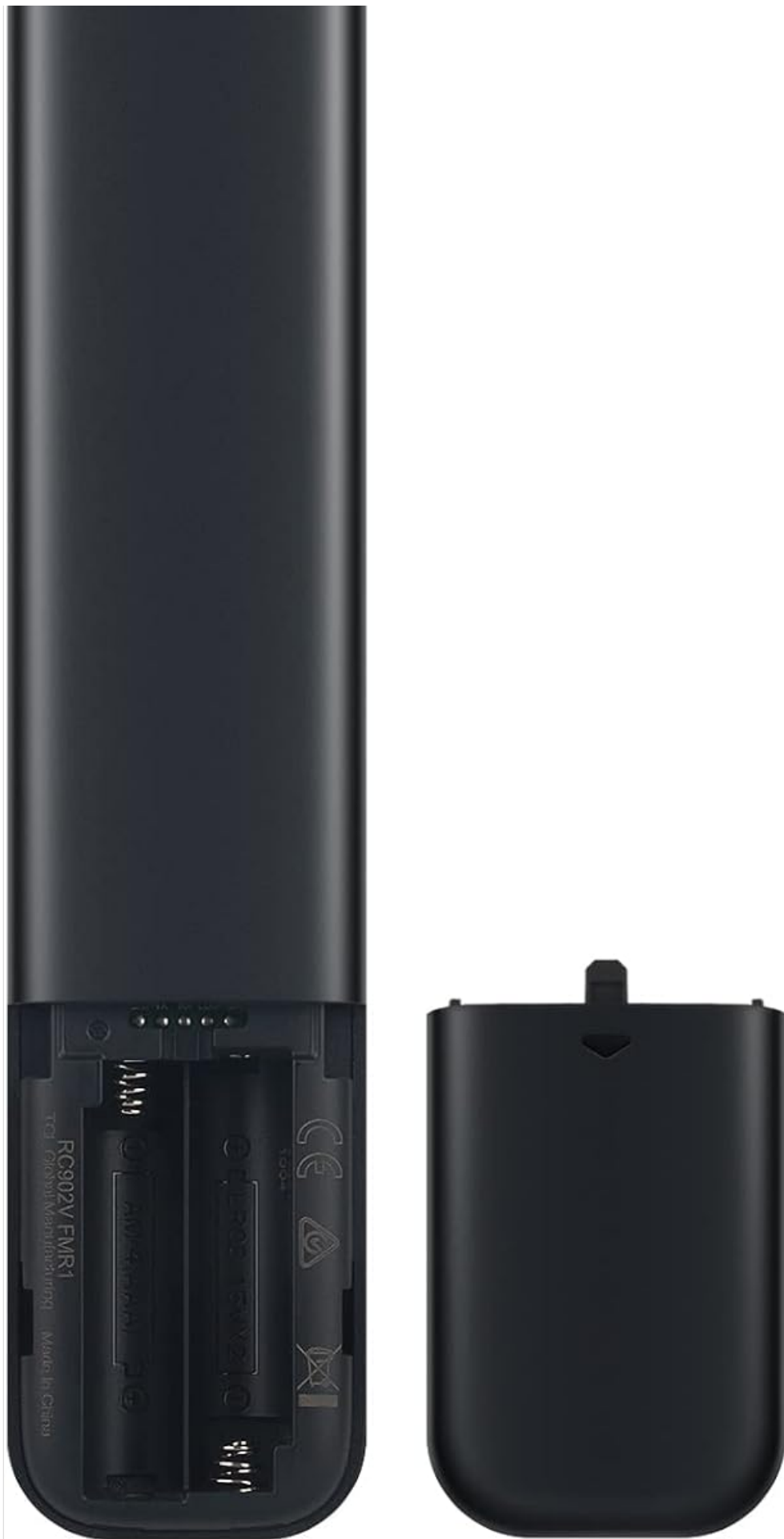
Image: Back view of the remote control with the battery cover removed, illustrating the correct orientation for AAA battery insertion.
