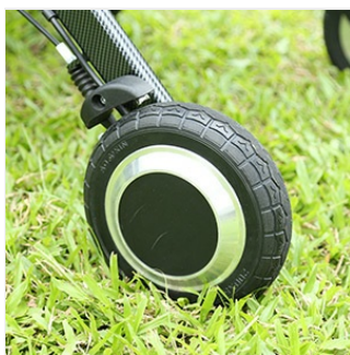
Figure 5.1: Detail of the brushless motor, requiring minimal maintenance.
