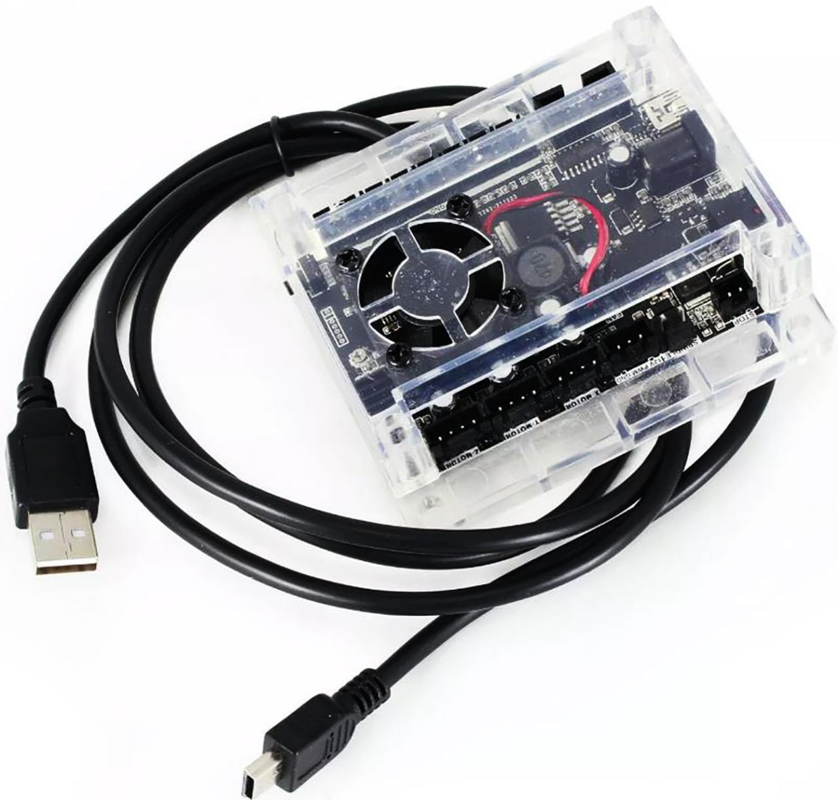
Image: The GRBL 1.1F 3-Axis Control Board with its accompanying USB cable.
