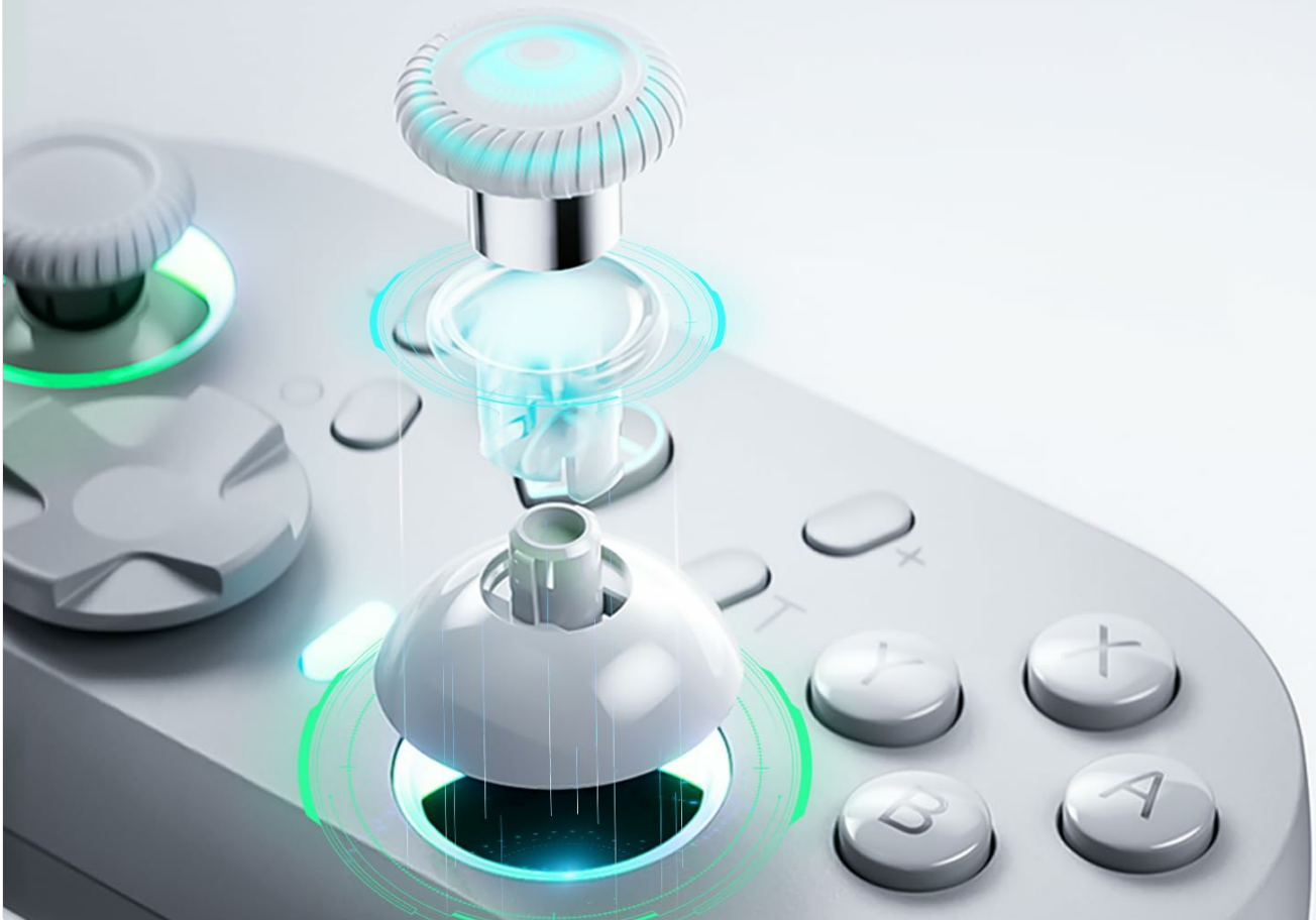
Figure 3: Diagram illustrating the Hall Effect sensing sticks for seamless, drift-free operation.
