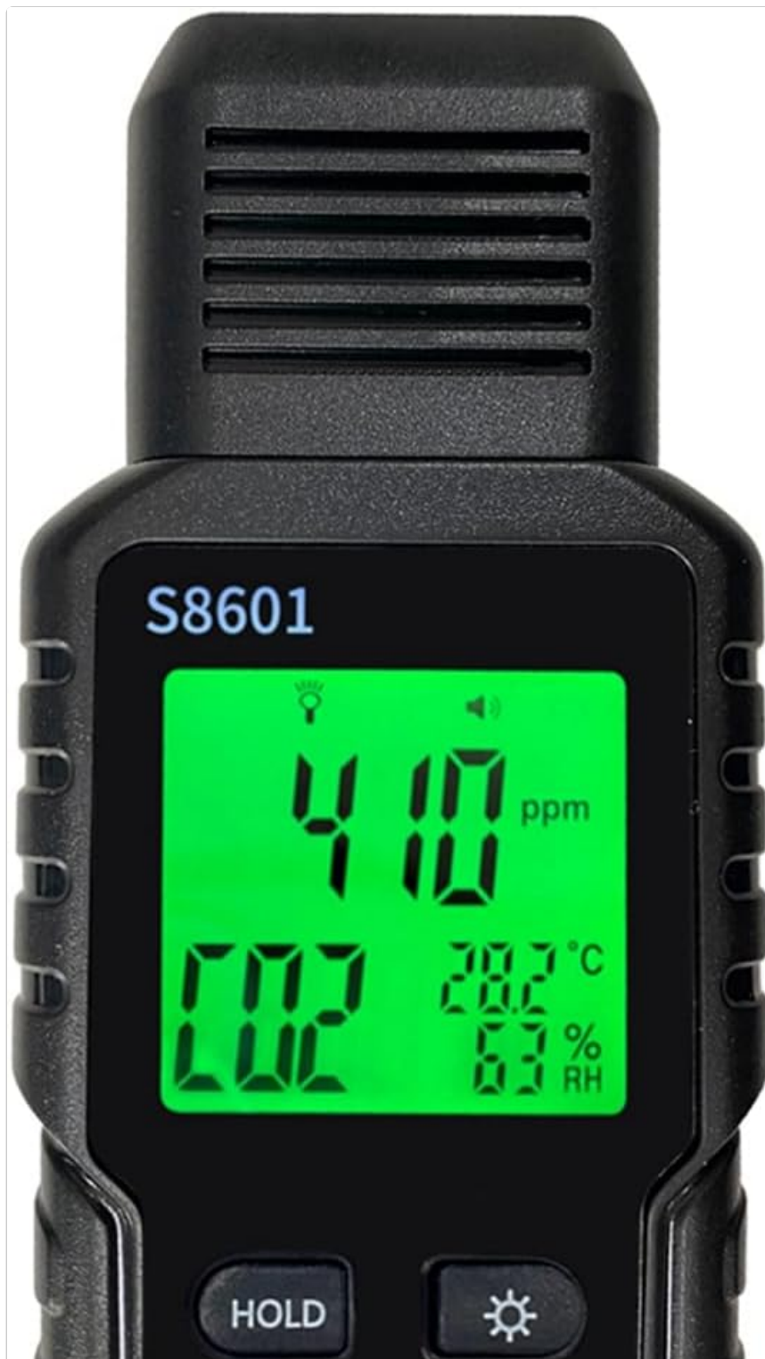
Figure 3.1: Front view of the Srutueo S8601A CO2 meter, displaying CO2 concentration (410 ppm), temperature (28.2°C), and relative humidity (63% RH).
