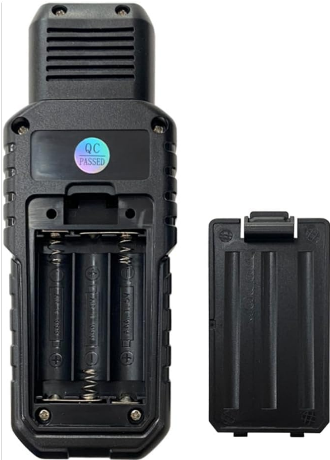
Figure 4.1: Battery compartment open, showing the correct placement for three AAA batteries.
