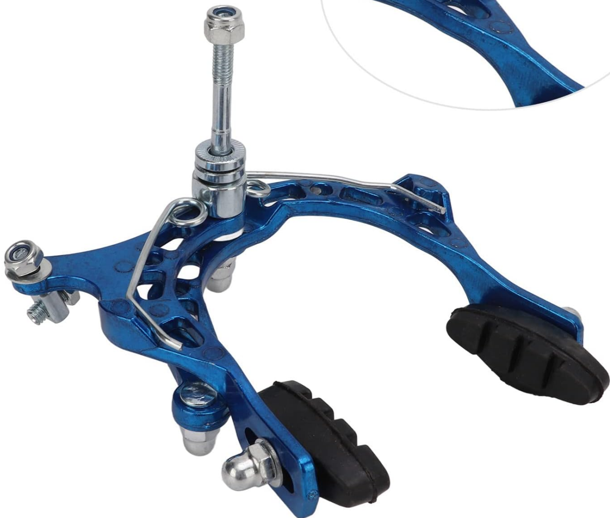
Figure 1: Close-up of the brake caliper, illustrating its robust construction and material quality. The image shows the blue aluminum alloy frame with black brake pads and silver mounting hardware.
