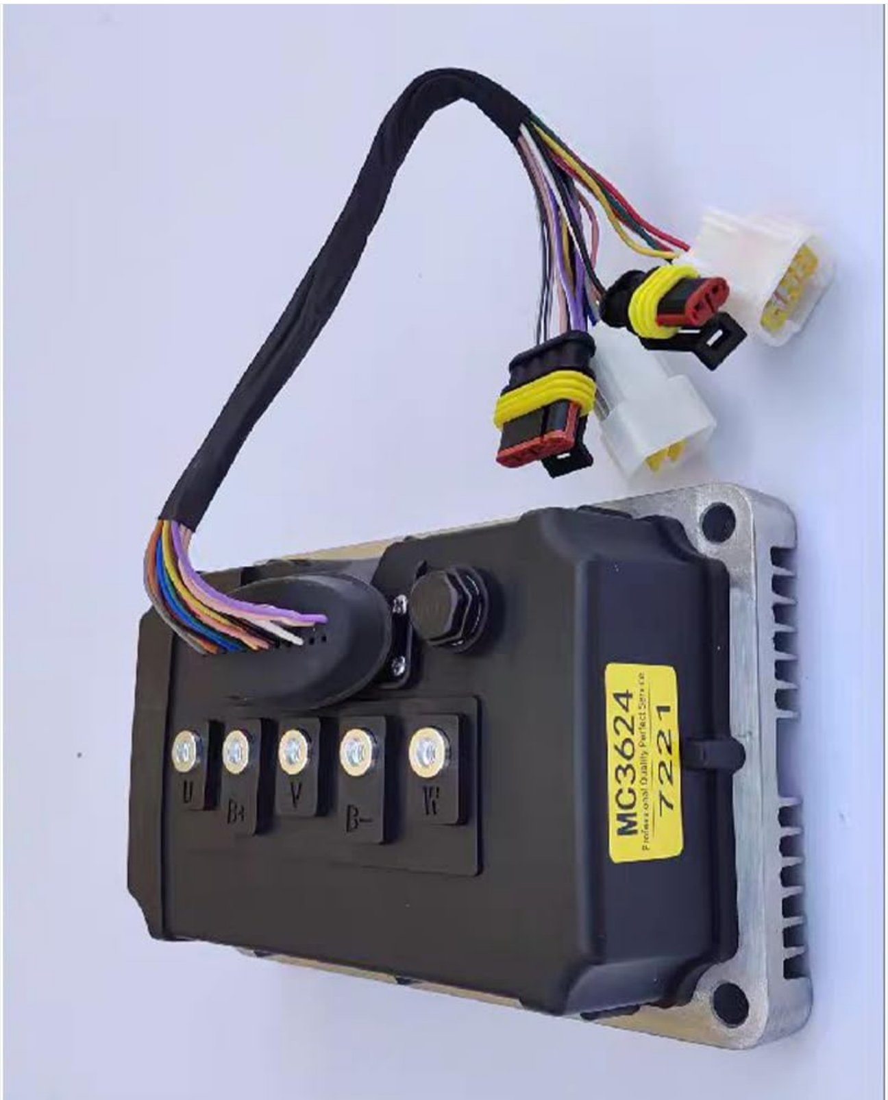
Figure 3: Side view of the Enpower MC3624 controller with its attached wiring harness, showing the various colored wires.
