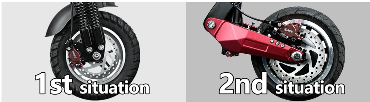
Image: Close-up of the brake caliper installed on a scooter wheel.
