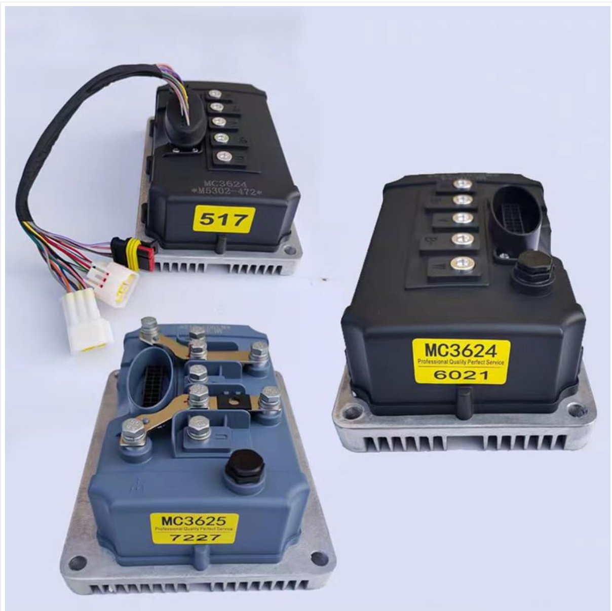
Figure 2: Side view of an Enpower MC3624 controller, highlighting the integrated wiring harness and the main connection terminals. This perspective helps in identifying the various input/output points.
