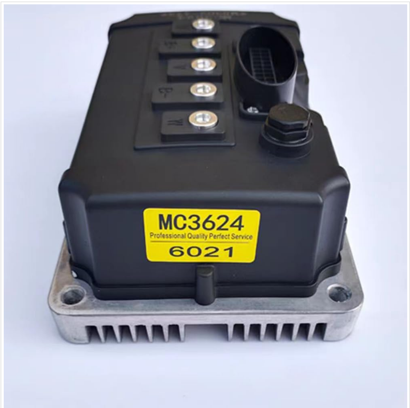
Figure 3.3: The Enpower MC3624-6021 controller, showing its specific model designation and connection points.
