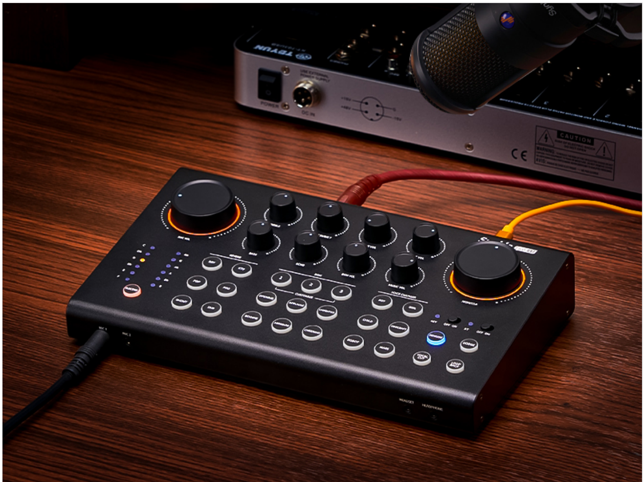
Image 2.1: Front Panel Controls. Key controls include Microphone volume, Volume adjustment buttons, Monitor volume, Electric sound switch, Reverb type, Warm-up sound effect, Voice changer, Phantom power switch, Function buttons, and BT switch.
