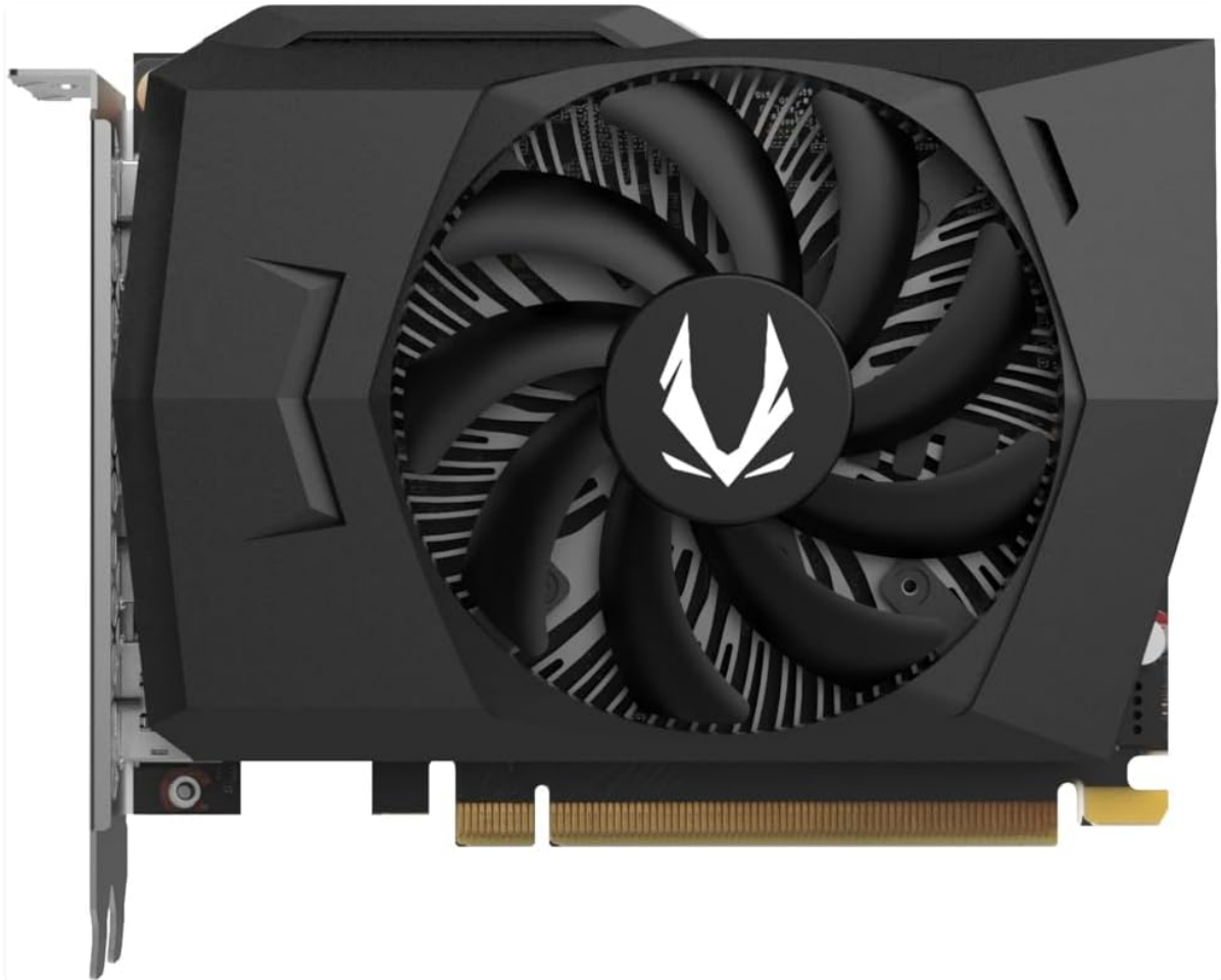
Figure 2: Top view of the ZOTAC Gaming GeForce RTX 3050 Graphics Card, showing the cooling fans.
