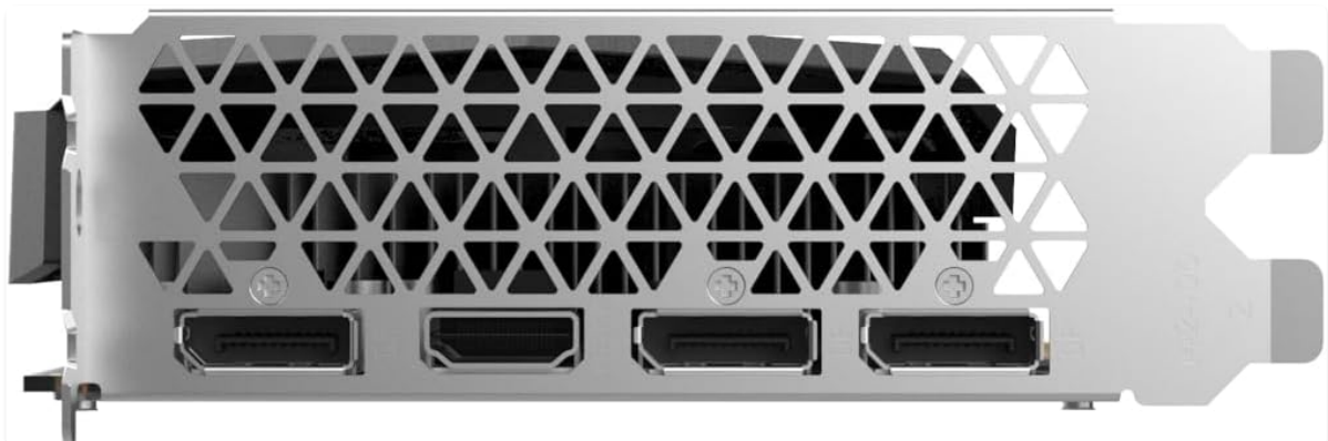
Figure 4: Rear view of the ZOTAC Gaming GeForce RTX 3050 Graphics Card, showing the DisplayPort and HDMI outputs.
