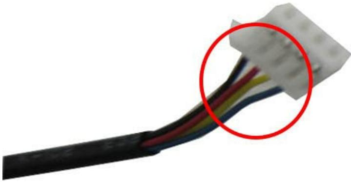
**Figure 1:** The 4-pin connector of the Mini PC Fan. Note the arrangement of the colored wires (red, yellow, blue, black) which is crucial for compatibility. Different wire sequences may exist, requiring careful verification before connection.
