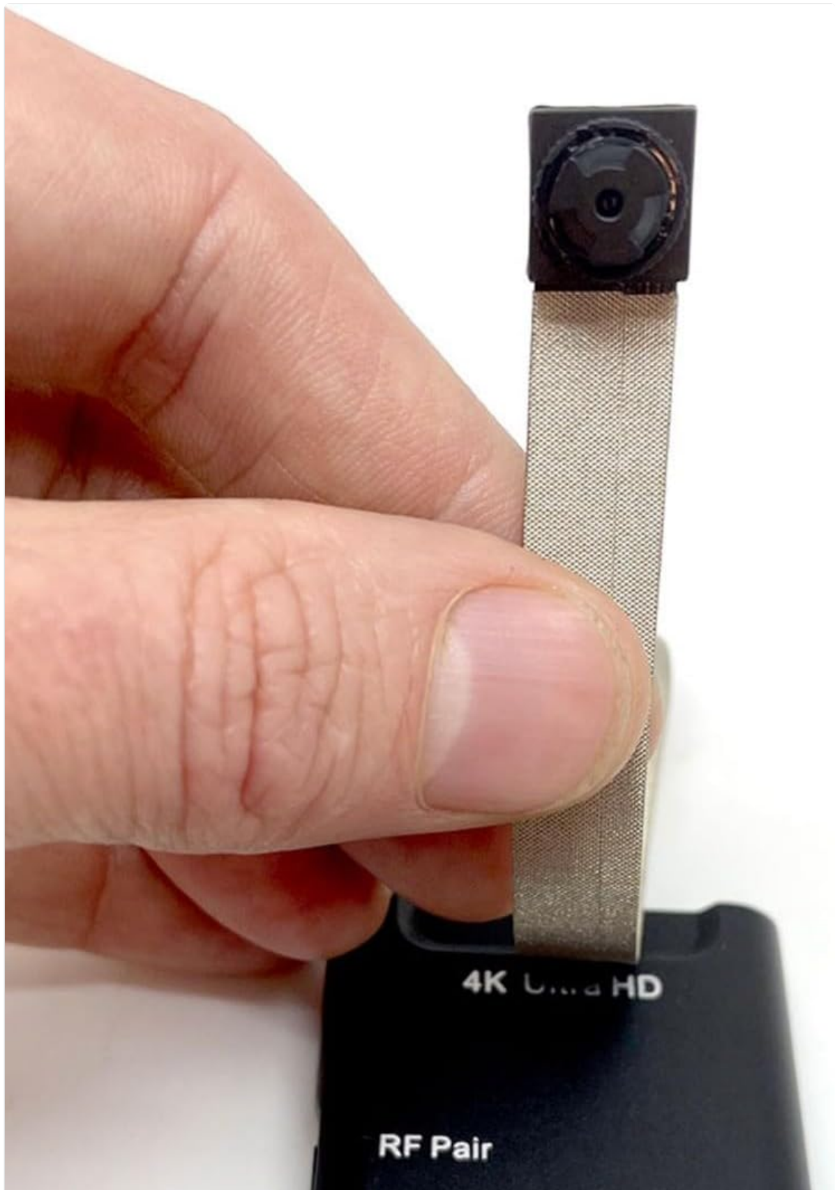
Image: The Lawmate PV-DY40UW DVR module, showing the main unit with the attached ribbon cable and pinhole camera. This view helps identify the components for setup.
