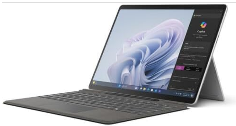
Figure 3.2: Side view of the Surface Pro 10 in laptop configuration, highlighting the adjustable kickstand and connected keyboard.
