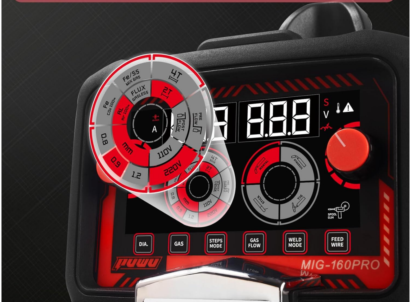
Image 4.3: The digital control panel of the PUWU MIG-160 PRO, illustrating how to change wire thickness or adjust amperage, with suggested voltage and wire transfer speed automatically switched.
