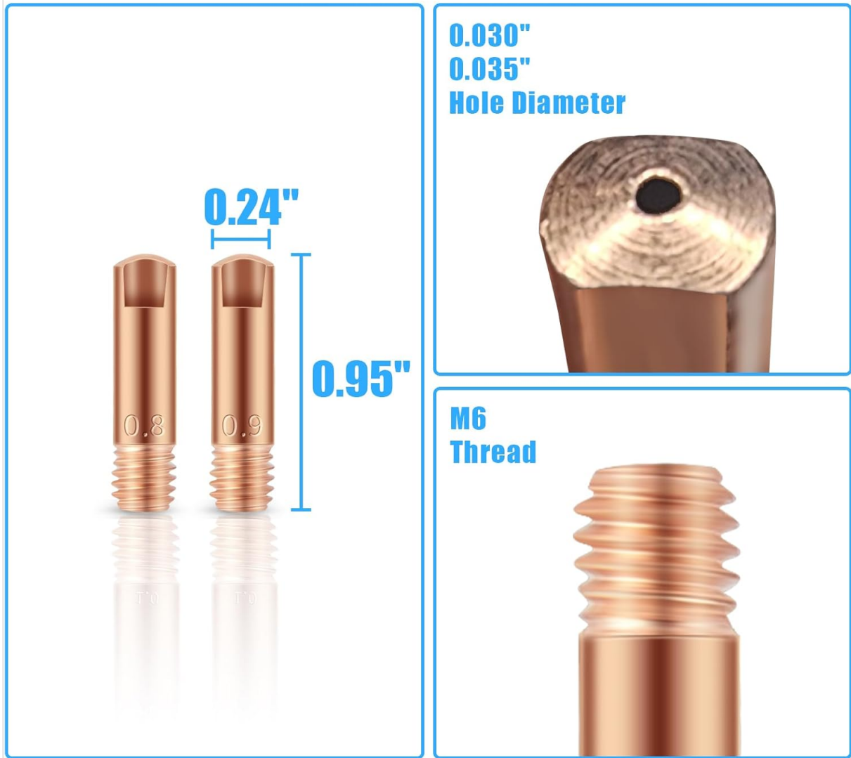
Image 3: Close-up of AZZUNO contact tips. The image highlights the dimensions, showing a length of 0.95 inches and a diameter of 0.24 inches. It also indicates a hole diameter of 0.030" or 0.035" and an M6 thread type.
