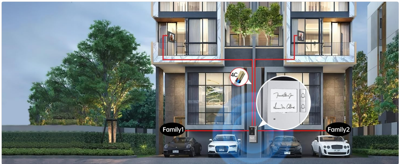
Figure 4.2: Various methods for unlocking the door: via the mobile app, using an RFID card, or directly from the indoor monitor.
