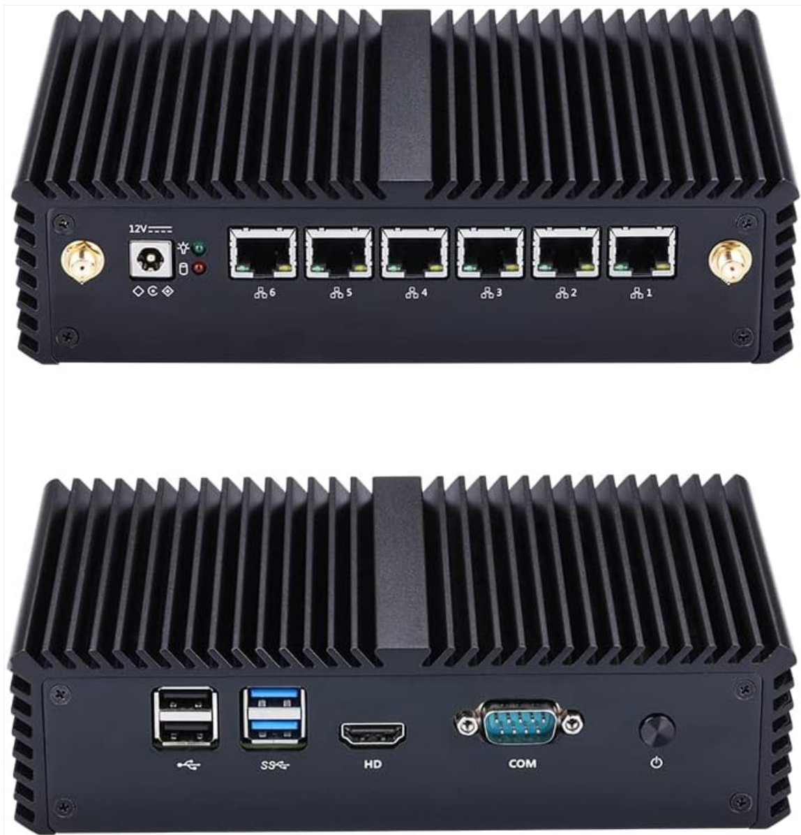
Figure 4.1: Front and Rear Panels of the Qotom Mini PC S05. The front panel includes the power input, power indicator, and six 1 Gigabit LAN ports. The rear panel features two USB 2.0 ports, two USB 3.0 ports, an HDMI port, a COM port, and the power button.
