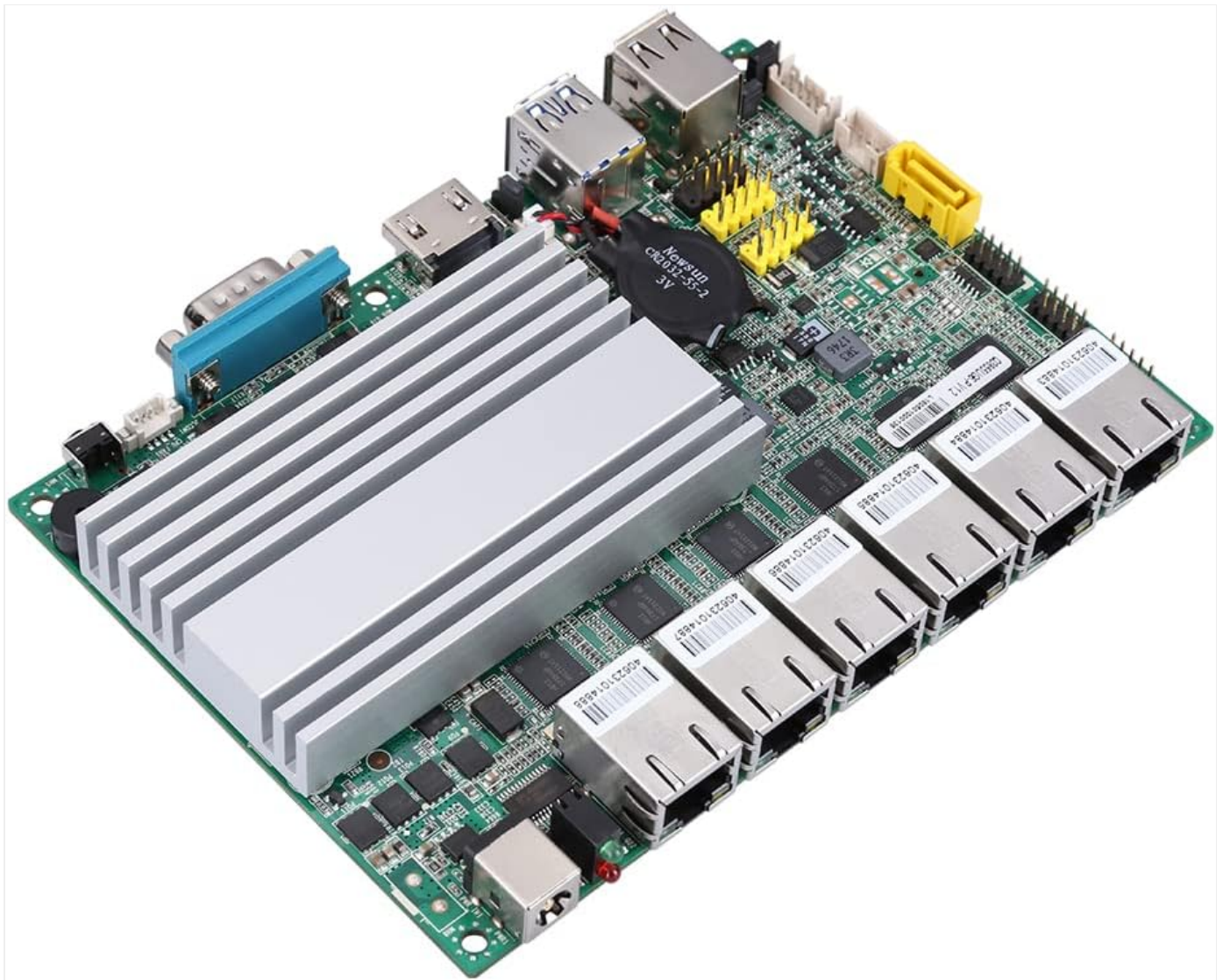
Figure 4.3: Detailed view of the Qotom Mini PC S05 motherboard, highlighting the Intel HD Graphics 620, various ports, and the heatsink for passive cooling. This image provides a closer look at the integrated components.
