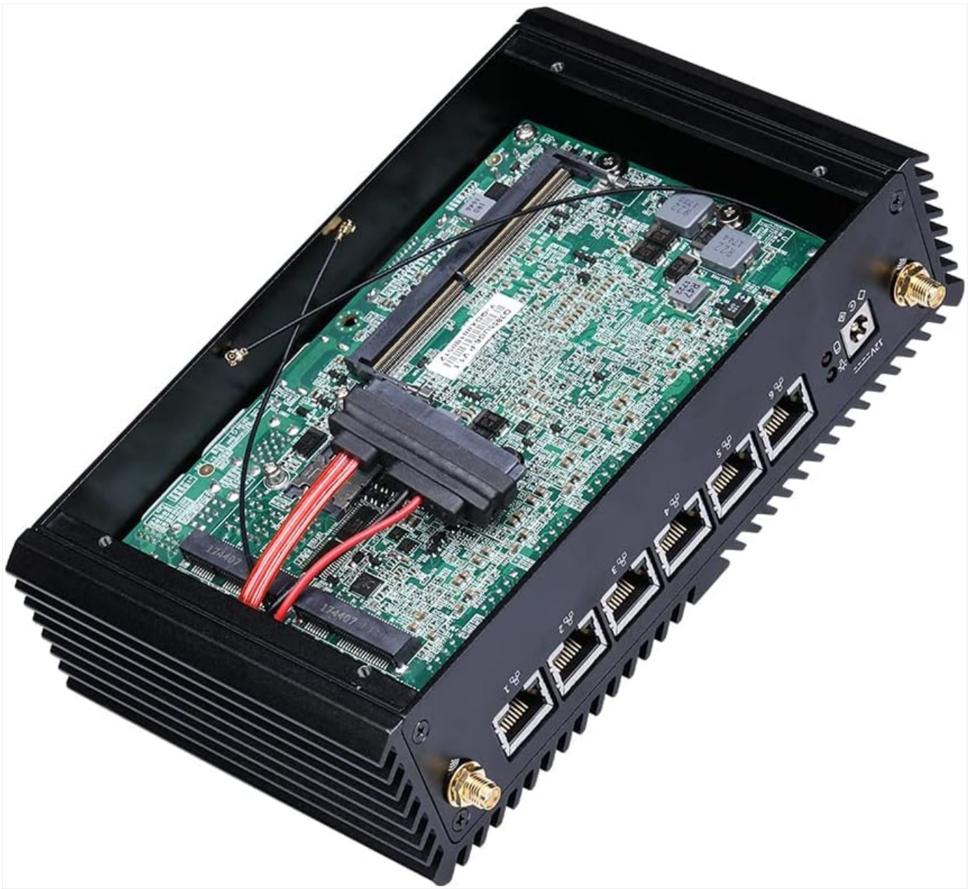
Figure 4.2: Internal view of the Qotom Mini PC S05, showing the motherboard, mSATA SSD slot, and RAM module. This view illustrates the compact and integrated design of the system components.
